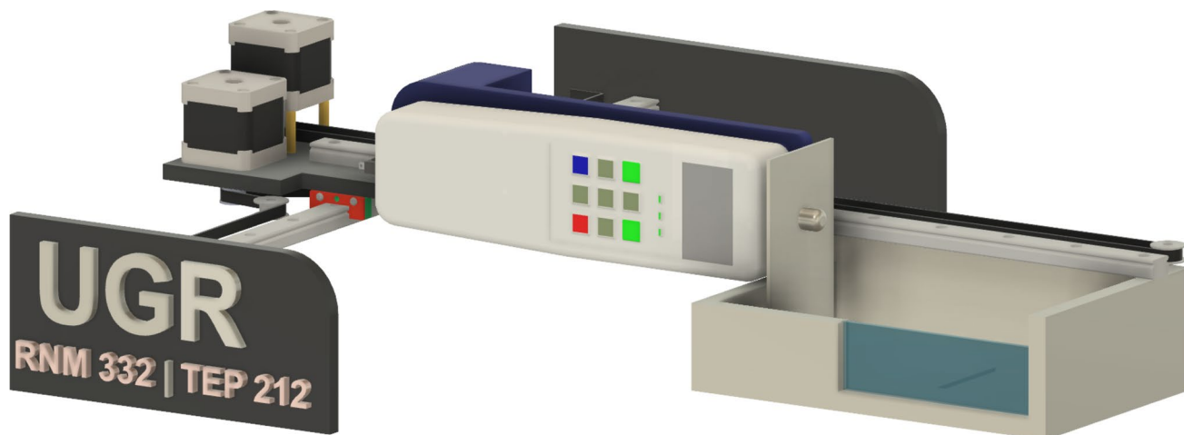
Fig. 3 Milli-manipulation device composed of (1) 2-axis displacement stage, (2) horizontal holder, (3) digital force gauge, (4) scraper, and (5) sample chamber
