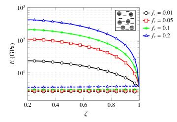
Figure 18: Macroscopic Young's modulus of Epon 862/EPI reinforced by fully aligned SWCNTs (5,5) with agglomeration parameter  $\xi$ =0.2 and varying agglomeration parameter  $\zeta$ . Solid and dashed lines denote longitudinal  $E_{\parallel}$  and transverse elastic moduli  $E_{\perp}$ , respectively.
