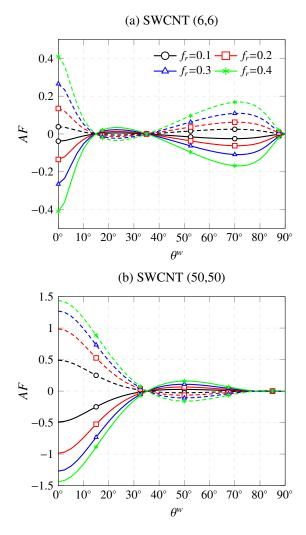
Figure 14: Asymmetry factors  $AF_{ij}$  as functions of the spiral angle  $\theta^w$  for helical CNT-reinforced Epon 862/EPI obtained using the MT approach with different SWCNT (6,6) (a) and SWCNT (50,50) (b) concentrations. Solid and dashed lines stand for  $AF_{12}$  and  $AF_{23}$ , respectively.
