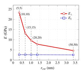
Figure 7: Longitudinal  $E_{\parallel}$  and transverse  $E_{\perp}$  Young's moduli of Epon 862/EPI reinforced by armchair SWCNTs versus CNT radius ( $f_r$ =0.01).
