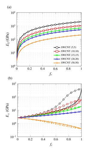
Figure 6: Effective Young's modulus in the longitudinal direction  $E_{\parallel}$  (a) and in the transverse direction  $E_{\perp}$  (b) versus filler volume fraction  $f_r$  of Epon 862/EPI reinforced by different aligned, straight SWCNTs (10,10), estimated by the MT and SC approaches, corresponding to solid and dotted lines, respectively.
