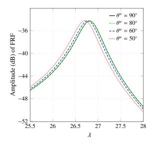
Figure 28: Frequency response function (FRF) plot of CNT/polymer skew plates with coupled waviness and agglomeration effects ( $f_r = 0.12, \xi=0.2, \zeta=0.4, a/b = 1, b/t = 50$ , SWCNT (5,5)).
