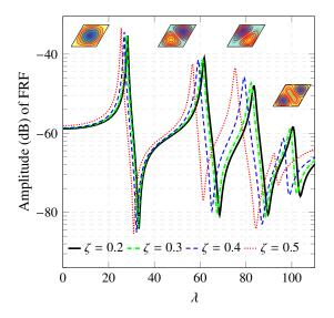
Figure 27: Frequency response function (FRF) plot of CNT/polymer skew plates with agglomeration effects ( $f_r = 0.12, \xi = 0.2, a/b = 1, b/t = 50$ , SWCNT (5,5)).
