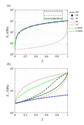
Figure 4: Effective Young's modulus in the longitudinal direction  $E_{\parallel}$  (a) and in the transverse direction  $E_{\perp}$  (b) versus filler volume fraction  $f_r$  of Epon 862/EPI cure W reinforced by aligned, infinitely long straight SWCNTs (10,10).
