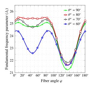
Figure 26: Effect of fiber angle  $\varphi$  on the first frequency parameter  $\lambda_1$  of CNT/polymer skew plates with waviness effects ( $\alpha = 60^\circ$ ,  $f_r = 0.12$ , a/b = 1, b/t = 50, SWCNT (5,5)).
