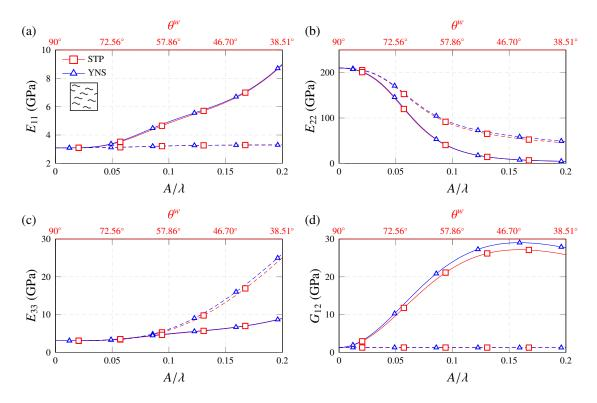
Figure 15: Elastic moduli predicted for Epon 862/EPI reinforced by fully aligned wavy SWCNTs (5,5) ( $f_r$ =0.1). Solid and dashed lines denote helical and planar sinusoidal configurations, respectively.
