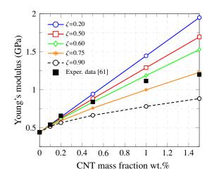
Figure 22: Comparison analysis of the macroscopic Young's modulus of SWCNT-nylon 6 composites considering randomly oriented straight dispersed fillers with agglomeration effects ( $\rho_r = 1.4 \text{ g/cm}^3$ ,  $\rho_m = 1.184 \text{ g/cm}^3$ , SWCNTs (10,10),  $E_m = 440 \text{ MPa}$ ,  $\nu_m = 0.2$ ,  $\xi = 0.2$ ,  $a_1 = a_2 = a_3$ ).
