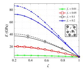
Figure 17: Macroscopic Young's modulus of Epon 862/EPI reinforced by randomly oriented SWCNTs (5,5) with agglomeration parameter  $\xi$ =0.2 and varying agglomeration parameter  $\zeta$ . Dashed and solid lines denote estimations by the MT and SPT approaches, respectively.
