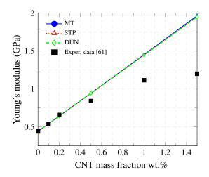
Figure 21: Comparison analysis of the macroscopic Young's modulus of SWCNT-nylon 6 composites considering randomly oriented straight uniformly dispersed fillers ( $\rho_r$ =1.4 g/cm<sup>3</sup>,  $\rho_m$ =1.184 g/cm<sup>3</sup>, SWCNTs (10,10),  $E_m$ =440 MPa,  $v_m$ =0.2).
