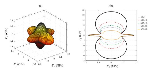
Figure 8: Surface contour of directional dependent Young's modulus ( $f_r$ =0.01, SWCNT (50,50)/Epon 862/EPI) (a) and planar projections on  $x_1$ - $x_2$  plane of Epon 862/EPI reinforced by armchair SWCNTs ( $f_r$ =0.01).
