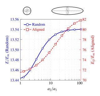
Figure 19: Effect of filler bundle aspect ratio  $(a_2/a_1)$  on the effective elastic properties of CNT-reinforced Epon 862/EPI Young's modulus of composites doped with randomly oriented CNTs, and longitudinal Young's modulus of composites doped with uniaxially aligned CNTs (SWCNT (5,5),  $\xi$ =0.2,  $\zeta$ =0.4,  $f_r$ =0.1).
