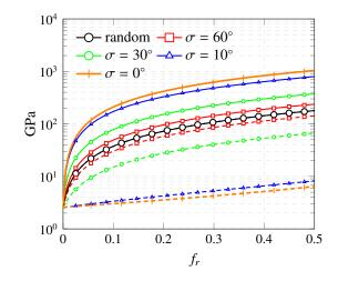
Figure 12: Elastic moduli as a function of volume fraction with different degrees of nanotube misalignment, for Epon 862/EPI reinforced by SWCNTs (5,5). Solid and dashed lines stand for longitudinal  $E_{\parallel}$  and transverse  $E_{\perp}$  Young's moduli.
