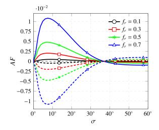
Figure 11: Asymmetry factor AF as a function of the orientation standard deviation  $\sigma$  for a symmetric truncated normal distribution obtained using the MT approach with different SWCNT (5,5) concentrations. Solid and dashed lines stand for  $AF_{12}$  and  $AF_{23}$ , respectively.
