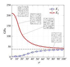
Figure 13: Longitudinal  $E_{\parallel}$  and transverse  $E_{\perp}$  Young's moduli as a function of orientation standard deviation  $\sigma$  of SWCNTs (5,5) with azimuthal symmetry ( $f_r$ =0.1).
