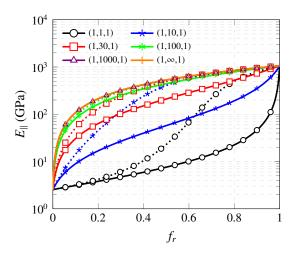
Figure 5: Effective Young's modulus in the longitudinal direction  $E_{\parallel}$  versus filler volume fraction  $f_r$  of Epon 862/EPI cure W reinforced by aligned, straight SWCNTs (10,10) with different aspect ratios, estimated by the MT and SC approaches, corresponding to solid and dotted lines, respectively.
