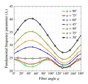
Figure 25: Effect of fiber angle  $\varphi$  on the first frequency parameter  $\lambda_1$  of CNT/polymer skew plates ( $f_r = 0.12, a/b = 1, b/t = 50, \text{SWCNT}(5,5)$ ).
