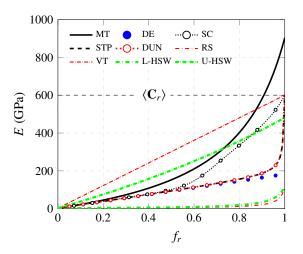
Figure 10: Young's modulus of Epon 862/EPI cure W reinforced by randomly oriented straight SWCNTs (10,10).
