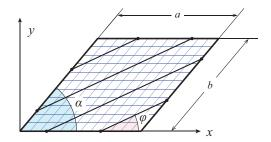
Figure 24: Geometry and configuration of CNT/polymer skew plates.
