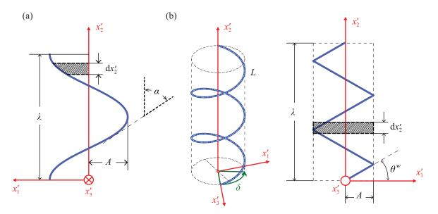
Figure 2: Planar sinusoidal (a) and helical model (b) of a curved CNT.
