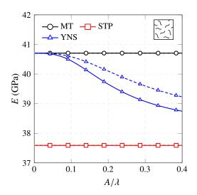
Figure 16: Elastic moduli predicted for Epon 862/EPI reinforced by randomly oriented wavy SWCNTs (5,5) ( $f_r$ =0.1). Solid and dashed lines denote helical and planar sinusoidal configurations, respectively.
