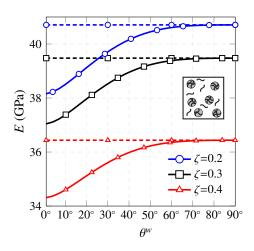
Figure 20: Macroscopic Young's modulus of Epon 862/EPI reinforced by randomly oriented wavy SWCNTs (5,5) with agglomeration parameter  $\xi$ =0.2 and varying agglomeration parameter  $\zeta$  as a function of the spiral angle  $\theta^w$  ( $a_1=a_2=a_3$ ,  $f_r=0.1$ ). Dashed lines denote the corresponding magnitudes for randomly oriented straight fillers.
