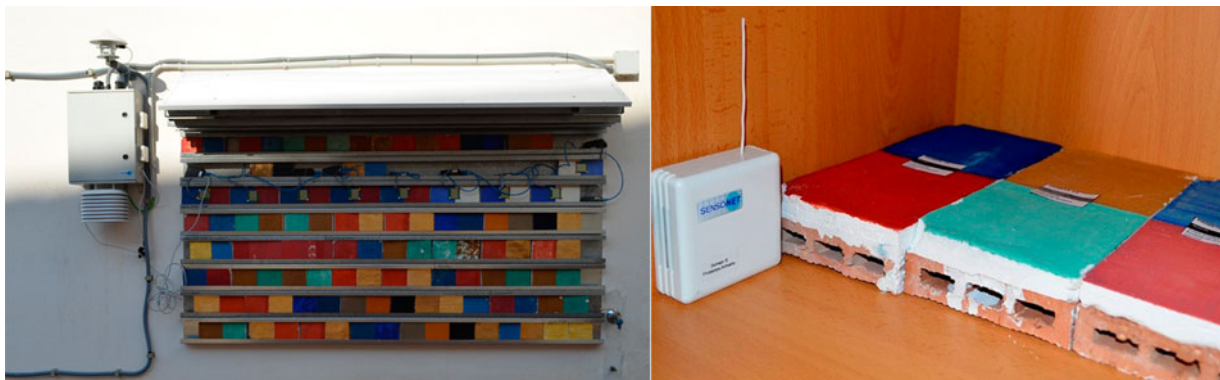
Figure 3. Left: General view of the samples exposed to outdoor ageing. Top left, the equipment for monitoring environmental conditions: pyranometer, anemometer, wind vane, ultraviolet sensor, temperature sensors, pluviometer, and relative-humidity sensors. Right: Detail of a few samples exposed indoors, showing the device controlling temperature and relative humidity.
