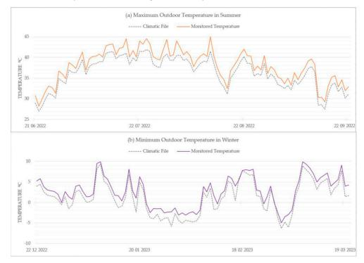
**Figure 3.** Thermal difference between the climatic data available from AEMET [81] and the monitored temperature. (a) Summer period with temperature differences due to the urban heat island effect. (b) Winter period with temperature differences due to the isolated building typology.
