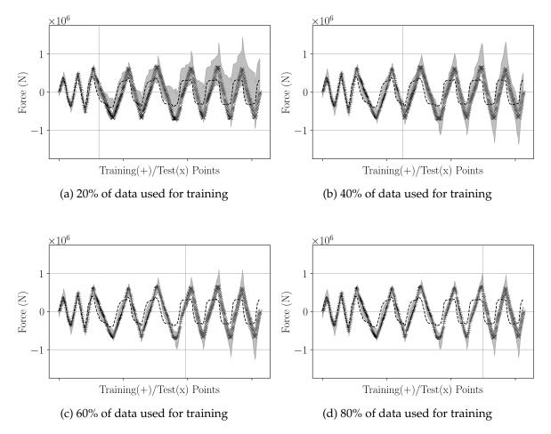
Figure 10.5: Data sensitivity analysis. The uncertainty quantified PG-BNN by ABC-SS (3) is represented by the grey hatch, the prediction of the physics-based model is given by the dashed line, the training data set is represented by '+' and the test data set is represented by 'x'. The vertical grey lines divide the training data domain from the test data domain. It can be seen how the uncertainty reduces gradually as more data is available for training.
