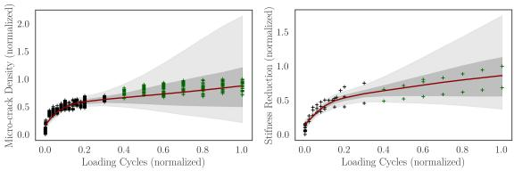
(a) Predictions of micro-cracks density.
