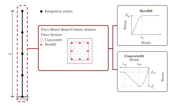
Figure 10.2: Schematic view of the nonlinear model of a cantilever reinforced concrete beamcolumn modelled using OpenSeespy. On the right-hand side, plots of the constitutive material monotonic behavior are presented.
