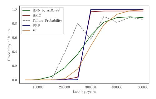
Figure 9.5: Evaluation of the probability of failure (0 to 1), based on the predictions made by the different Bayesian Neural Networks. The threshold for plausible failure was set at 0.8 micro-crack density (normalized).
