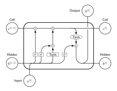
Figure 4.4: Generic diagram of Long Short Term Memory neural networks (by J. Leon).
