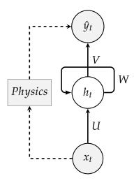
Figure 7.1: Schematic representation of the folded Physics-guided BRNN by ABC-SS
