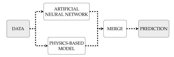
Figure 4.2: Generic diagram of physics-guided artificial neural networks
