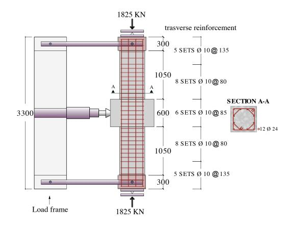
Figure 10.1: Double-ended reinforced concrete beam-column specimen details, adapted from [2].
