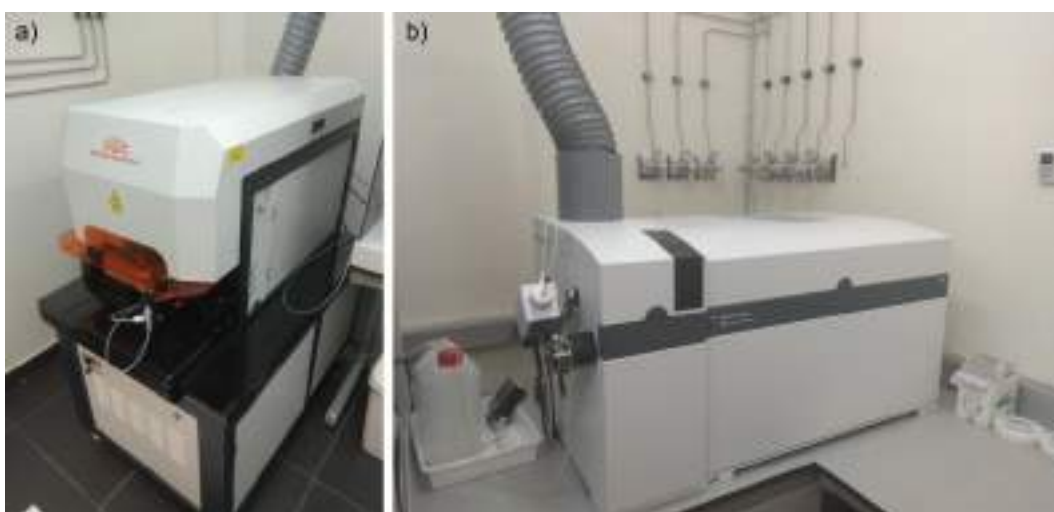
Figure 3.3. Photon Machine Analyte G2 laser ablation system (a) coupled to an Agilent 8800 QQQ inductively coupled-plasma mass spectrometer (b) at the facilities of the Instituto Andaluz de Ciencias de la Tierra (CSIC-Universidad de Granada, Spain).
