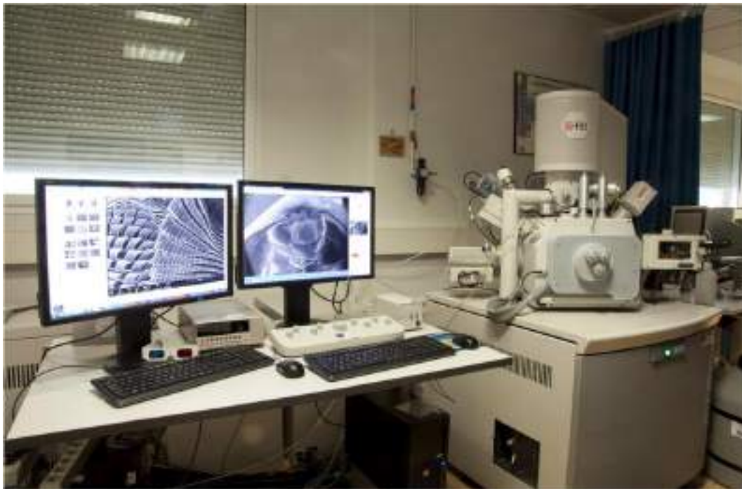
Figure 3.1. Field emission gun environmental scanning electron microscope (FEG-ESEM) at the Centro de Instrumentación Científica (CIC) of the Universidad de Granada (Spain).
