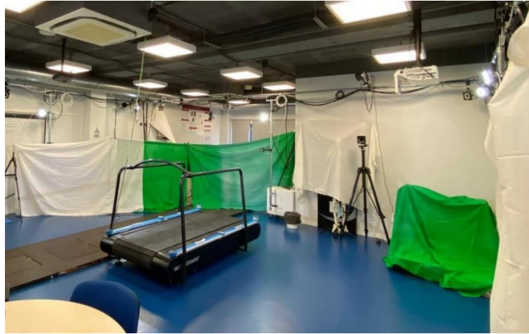
Figure 23. Image of the HumanLab with the treadmill centred, the photocell system placed on the treadmill, and the ring of 8 cameras placed on the bars around the lab with the LED light on.
