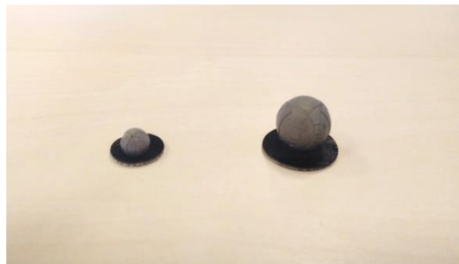
Figure 21. Image of the passive reflective markers used, 6mm diameter marker (left) and 12mm diameter marker (right).
