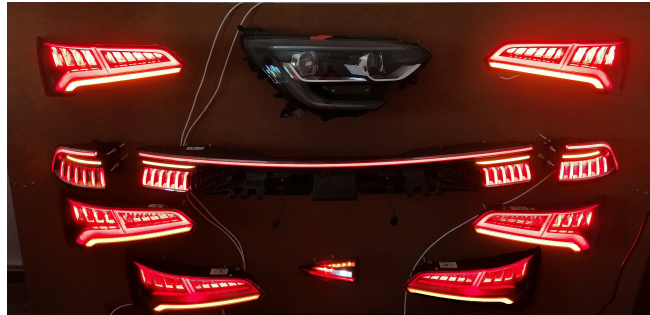
Video 3.2 – Controlling Audi Q8 2018 pilots with Audi “ Rearlamps Management v1.1.13 ”
