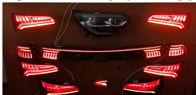
Video 3.1 – Setup for Audi Q8 2018 pilots controlling and sniffing
