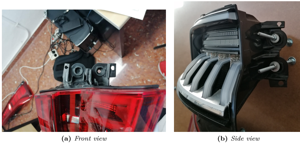
Figure 4.52 – Anchoring method of Fender light of Audi Q8 2018
