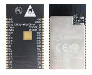
(f)  $Espressif \quad ESP32\text{-}WROVER\text{-}x$ series package. Extracted from: [96].
