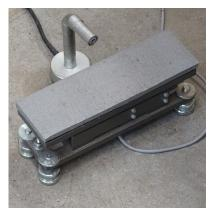
(g) PLG's microphone and load cell.
