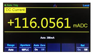
(a) LCD-only average power consumption measured with a Siglent SDM3065X digital multimeter.
