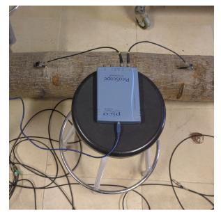
(a) Measurements in log with the Picoscope 4424.
