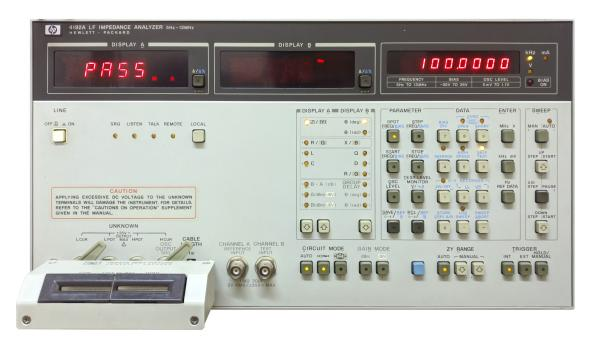
Figure F.16 – Front panel of the HP4192A LF impedance analyzer in the L-4 laboratory of the Faculty of Sciences; with the 16047A test fixture coupled.
