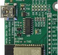
(b) Detail of the USB circuit after repositioning the ferrite bead.
