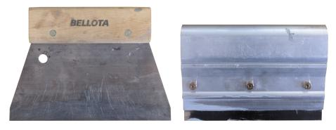
(c) Spatulas used to spread the solder paste on the stencil.
