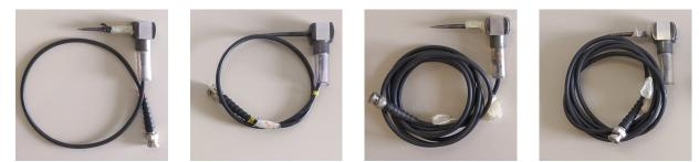
(a) Probe  $N^{\varrho}1$ , with 50 cm (b) Probe  $N^{\varrho}2$ , with 50 cm (c) Probe  $N^{\varrho}4$ , with 200 cm (d) Probe  $N^{\varrho}5$ , with 200 cm long cable. long cable.
