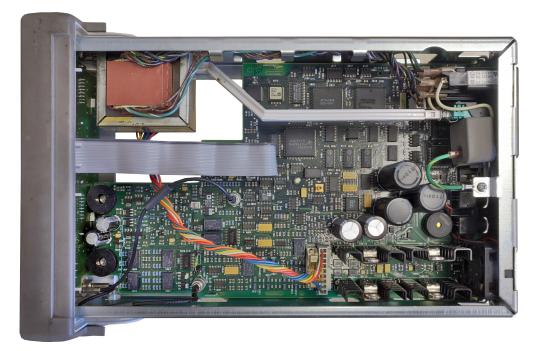
Figure F.5 – Photo of the internals of the HP33120A.
