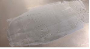
(e) Stencil with solder paste spread.
