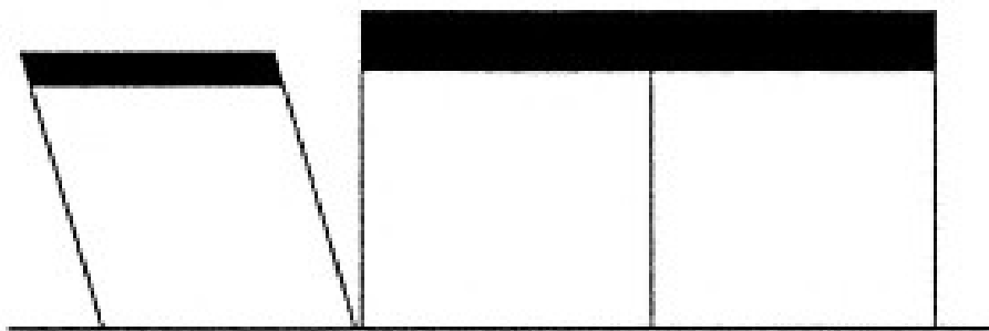
(b) Heavier Adjacent Building Pounding
