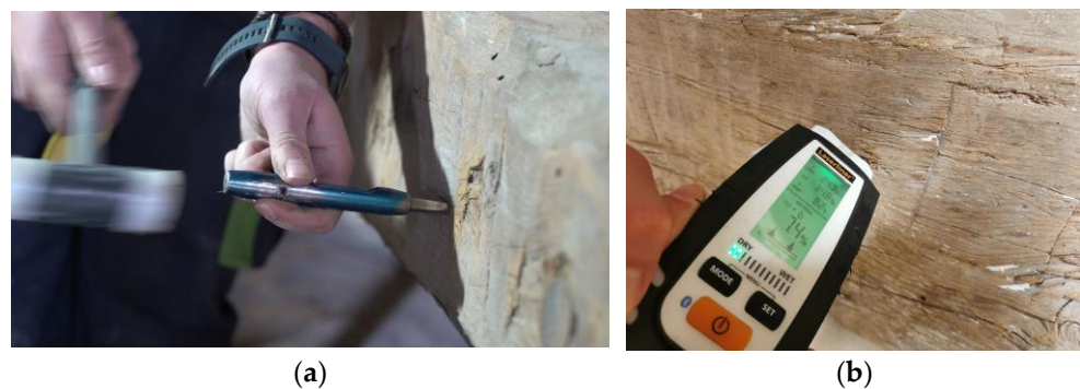
Figure 9. (a) Micro-core extraction using the Trephor35 auger. (b) Measurement of the moisture content of a beam using a hygrometer.
