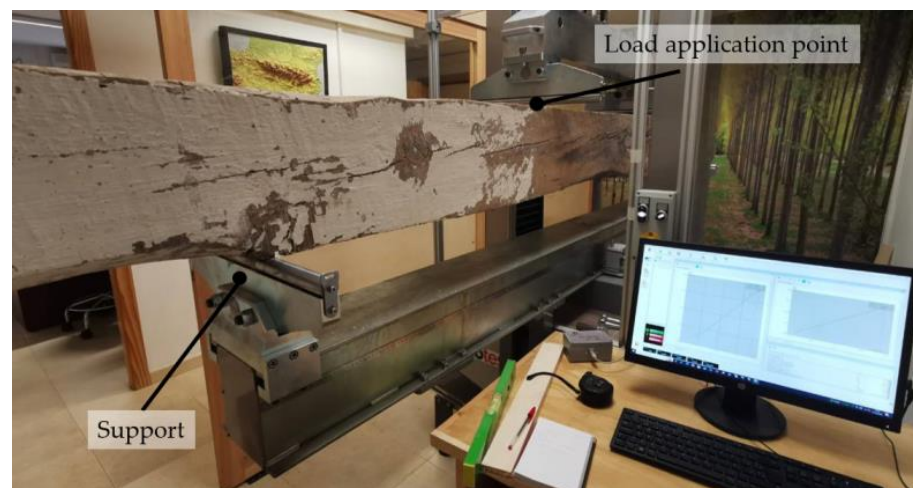
Figure 10. Beam subjected to four-point bending test.
