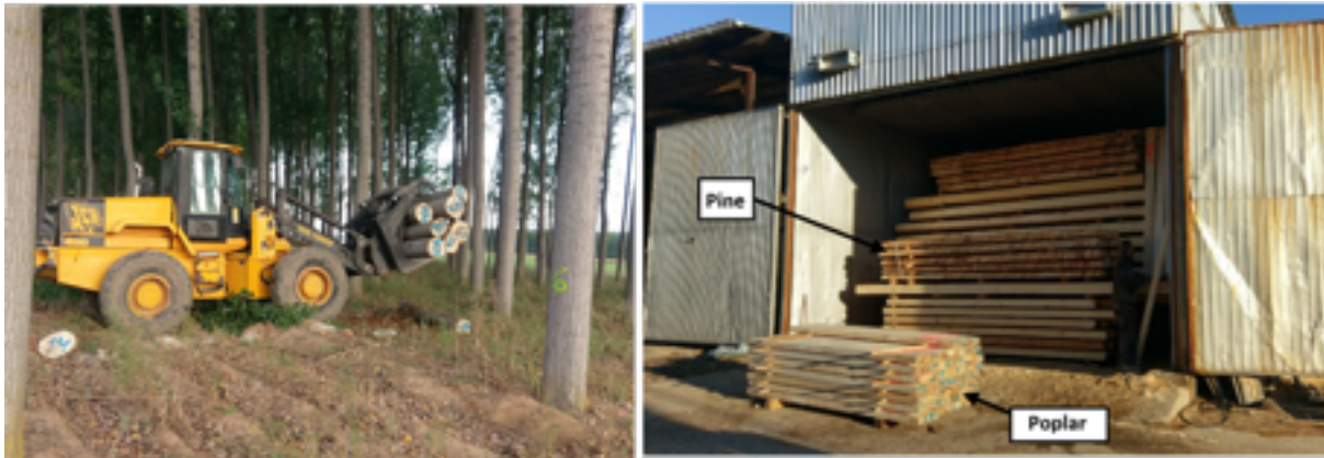
Figure 2.2: Left: Works during poplar harvesting; Right: Pine and poplar timber in the artificial dryer once the final MC=12% was achieved
