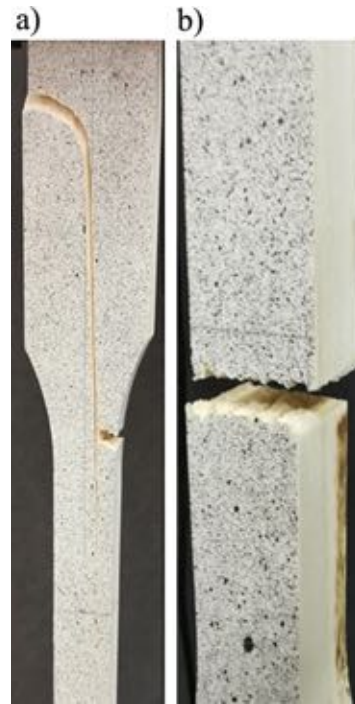
Figure 7.8: Modulus of elasticity variation of the specimens with finger joints-TF (left) and without finger joints-TT (right).
