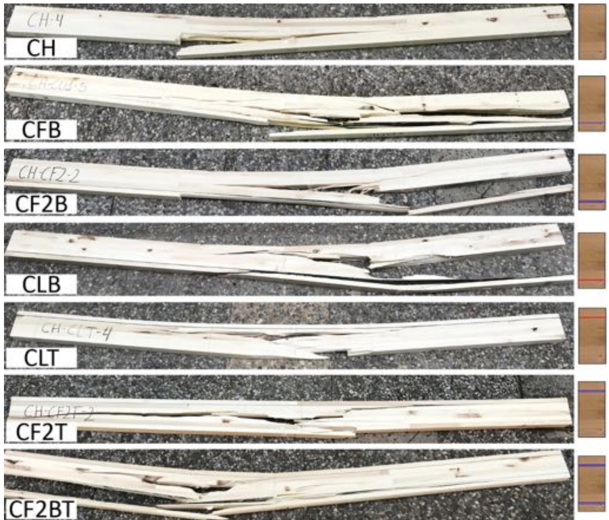
Figure 4.10: Failure patterns of the specimens.
