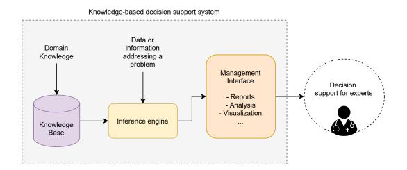
Fig. 2.2.: Architecture of a knowledge-based decision support system.
