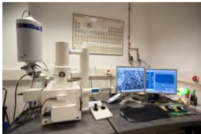
Figure 2. Variable Pressure Field Emission Scanning Electron Microscope (VP-FESEM) Zeiss SUPRA40VP equipped with SE (InLens) and BSE detectors. This microscope is located at “Centro de Instrumentación Científica” in the University of Granada ( https://cic.ugr.es/servicios-y-unidades/ficha.php?codServicio=6&unidad=49 ).
