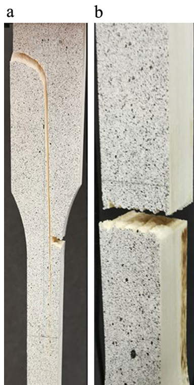
Fig. 8 Failure pattern of the TT (a) and TF (b) specimens
