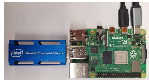
FIGURE 7. Recording setup for the offline proof-of-concept of the system generalization capability at the edge. The Raspberry® Pi4 is used for data preprocessing, model adaptation and script running. The NCS 2 enables the deployment of the developed meta-learning model for a specific setup.
