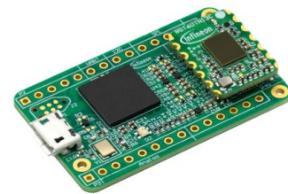
FIGURE 3. BGT60TR13C Radar System. The radar sensor, is mounted on top of the board.
