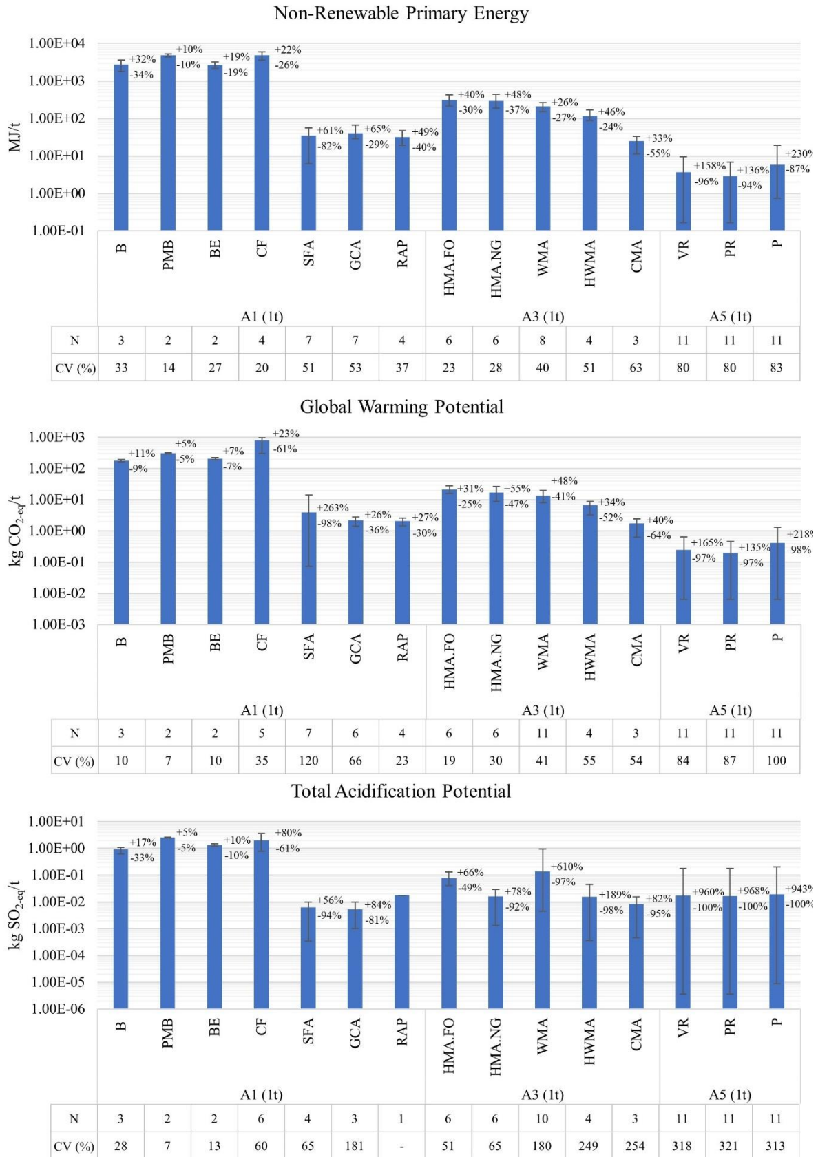
Figure 4.8. Logarithmic plot of PENRE, GWP, and TAP impact categories for the A1-A5 stages analysed with upper and lower bounds.
