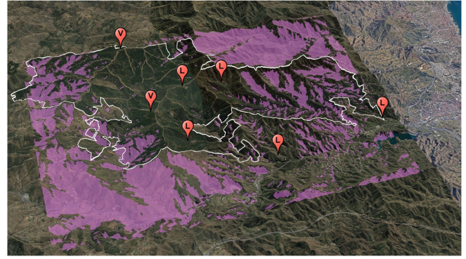
Fig. 4. CHAR map generated at the end of Stage-2. It shows the remaining uncovered area (purple layer) after having analyzed the viewshed from the initial five logistic points (L) and two points of maximum viewshed ( V ) in W_p . The white line represents the boundaries of the Montes de Malaga Natural Park.
