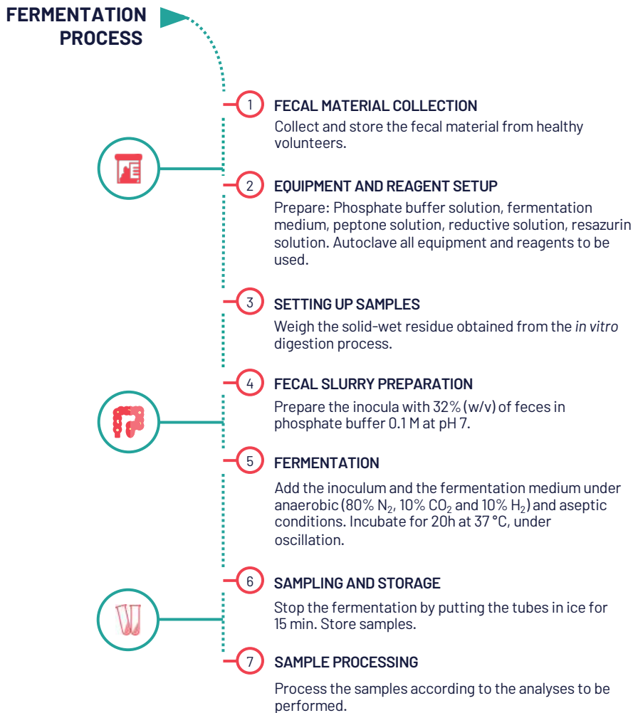
Figure 3.1.2 Scheme of the fermentation process.
