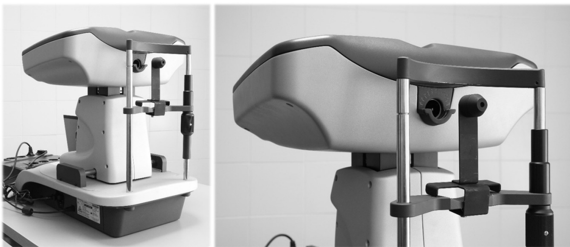
Figure 6. Artificial eye fixed to the OQAS device to measure optical quality.
