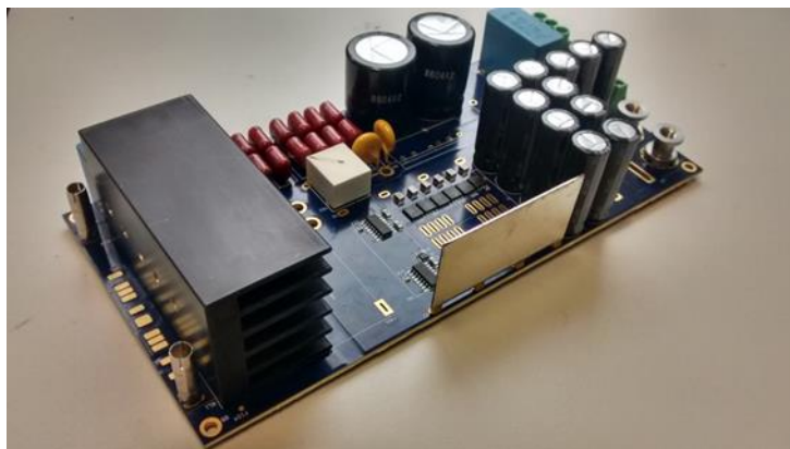
Figure 24. Heatsinks for HV half bridge bridge devices and LV secondary devices in a partially assembled 3300 W HB LLC converter board.
