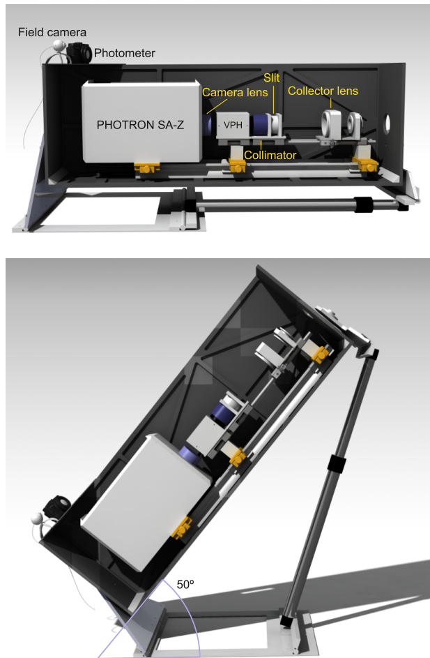
Figure 4.2: GALIUS mechanical housing
