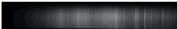
Figure 4.3: Spectral image of a deuterium lamp recorded with GALIUS for grism R1 using the collector lens D (50 mm focal length).
