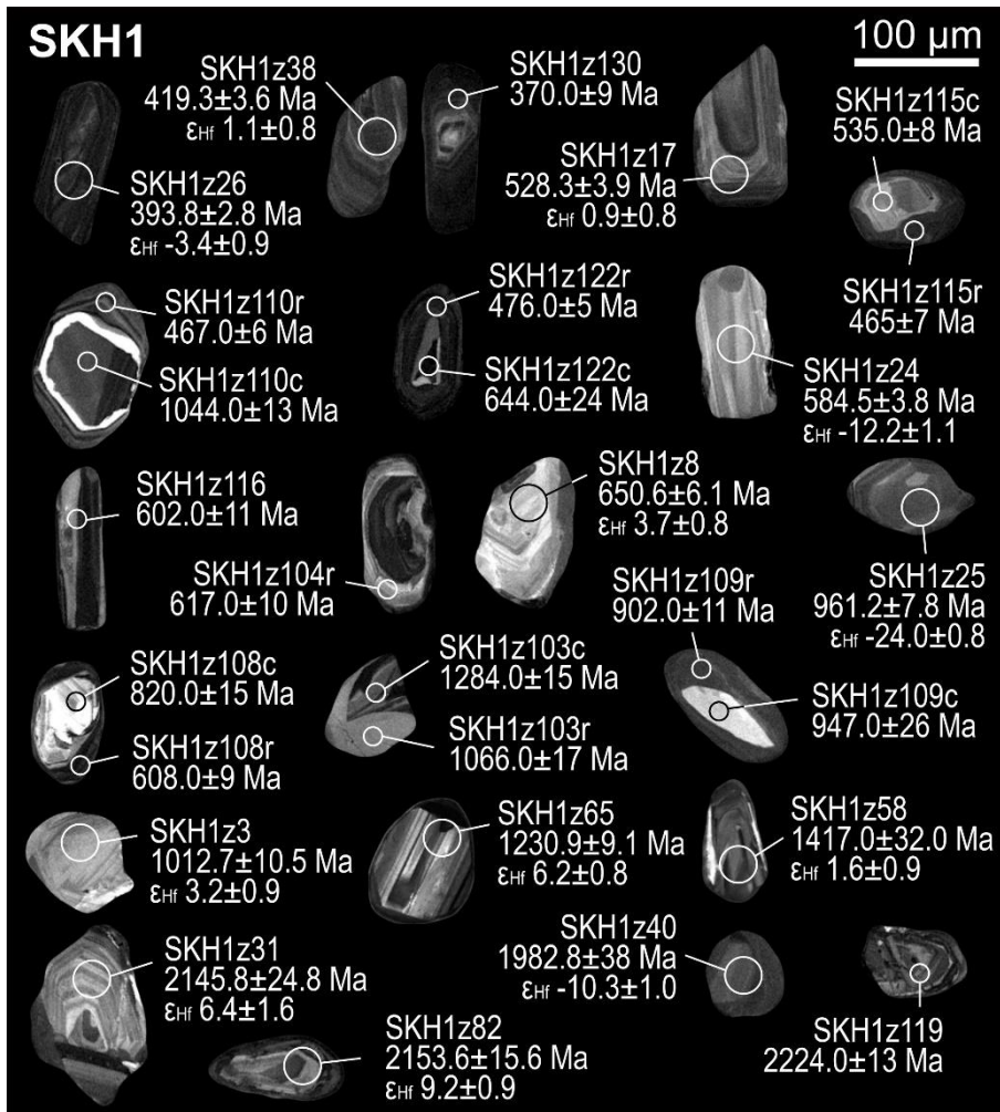
Figure C.19. Cathodoluminescence images of selected detrital zircon grains from the Visean sample SKH1 (IGSN: IEACC0011), accompanied by the result of the corresponding U-Pb analyses and, when available, Hf analyses.
