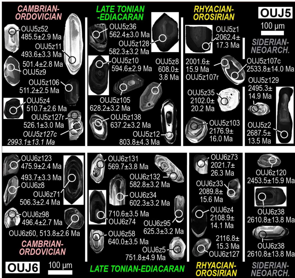
Figure C.11. Cathodoluminescence images of selected detrital zircon grains from the Early-Middle Ordovician samples OUI5 (IGSN: IEACC0021) and OUI6 (IGSN: IEACC0022), accompanied by the result of the corresponding U-Pb analysis.
