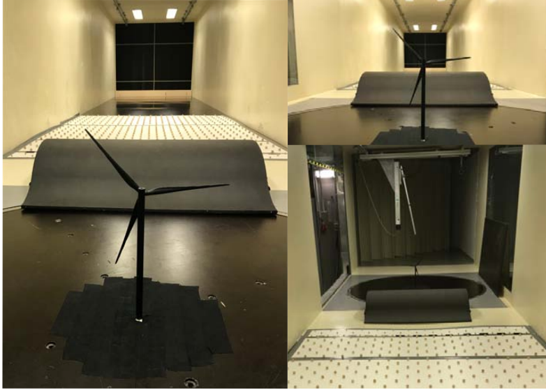
Figure 4.15: Set up, hill, and wind turbine models used for tests the CCWT.
