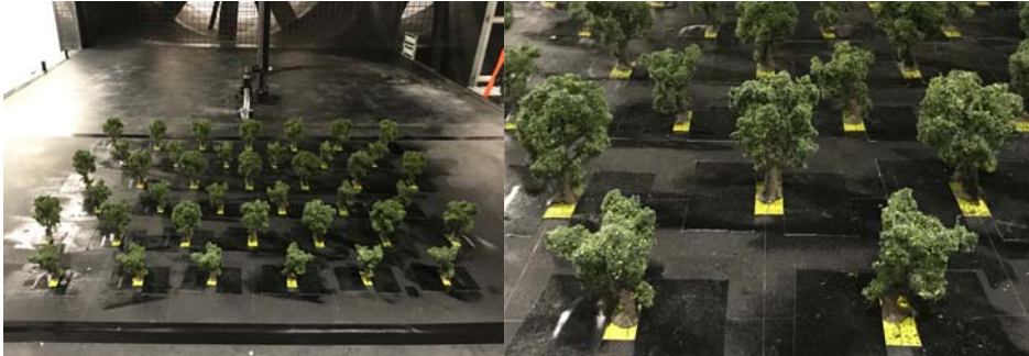
Figure 3.5: Images of staggered olive grove configuration (traditional olive grove without vegetation cover, C2).
