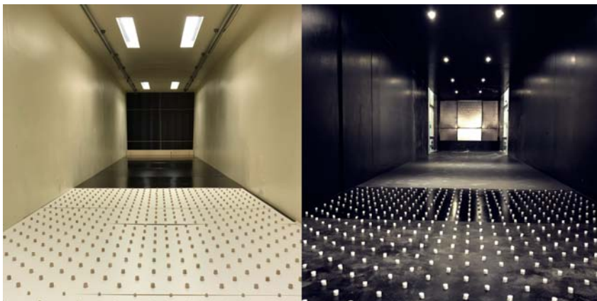
Figure 4.17: ABL simulated with roughness elements inside the CCWT (left) and the OCWT (right).
