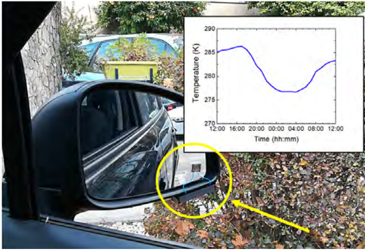
Figure I.8: Temperature sensing solution integrated in the side-view mirror of a car. Inset shows the temperature recorded during one day.
