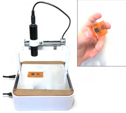
Figure II.1: Experimental setup for the laser irradiation of the polyimide surface. The inset displays a sample with two patterned areas of 1 \text{ cm}^2 on the surface scribed at two different values of the laser power: 50 mW (lighter one) and 100 mW (darker one).
