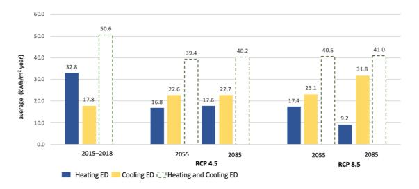
Figure 42. Dynamics of changes in the average of heating and cooling energy demand for the RCP4.5 and RCP8.5 scenarios by 77 station.
