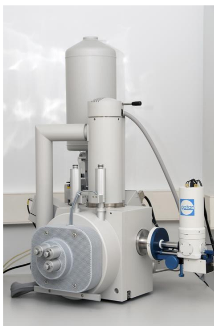
Figure 2. Environmental scanning electron microscope from “Centro de Instrumentación Científica” of the University of Granada.
