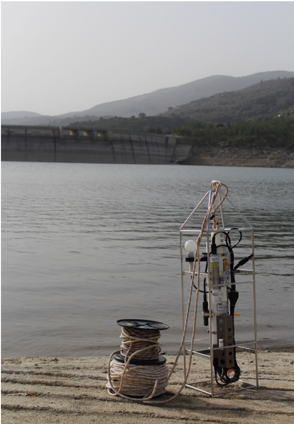
Figure 2.10. Sea-Bird 19 plus CTD profiler in the Bézinar reservoir.
