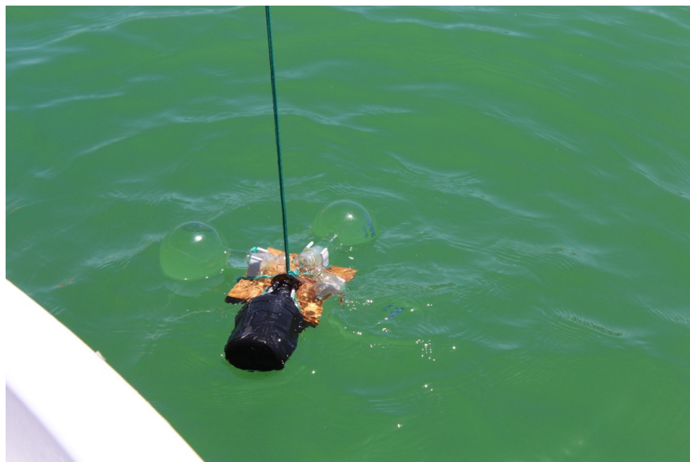
Figure 2.15. Incubation of quartz bottles during the photochemical experiments in the Cubillas reservoir.
