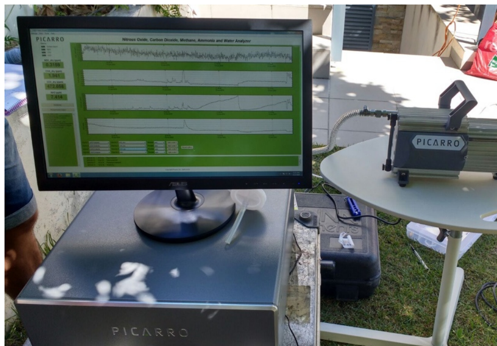
Figure 2.6. A picture of the Picarro G2508 analyzer including the monitor, and the vacuum pump.
