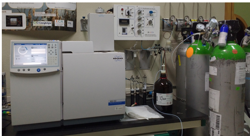
Figure 2.12. Gas chromatograph Bruker® GC-450 at the Department of Physical Chemistry at the University of Cádiz
