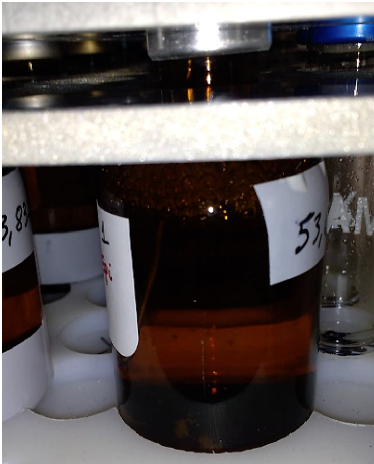
Supplementary Figure 7.5. Picture of an incubation bottle, where the suspended particulate material can be seen.
