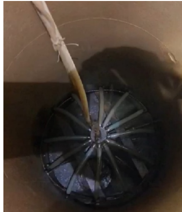
Figure 6. PVC diffusers at the bottom of a column.
