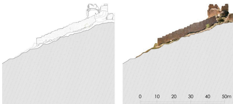
Figure 6. Orthophotography and planimetry of the east elevation of Lojuela Castle, located on the promontory. Source: PREFORTI project.
