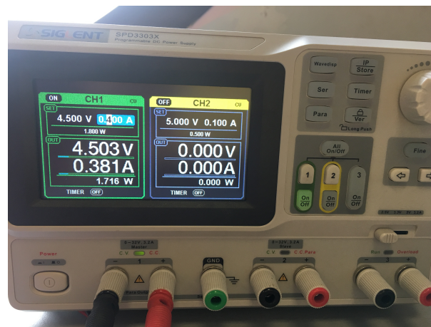
Figure 6.20 – LED Power consumption
