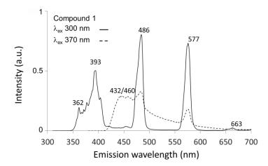
**Figure 10.** Room temperature solid state emission spectra of **1** upon sample excitation at  $\lambda_{ex} = 300$  nm (solid line) and  $\lambda_{ex} = 370$  nm (dashed line).
