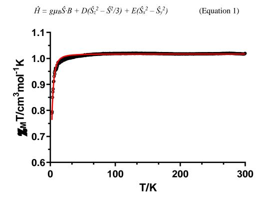
**Figure 6.** Temperature dependence of the  $\chi_M T$  product for compound 1 in the 2.5-300 K range. The solid line is generated from the best fit to the magnetic parameters.
