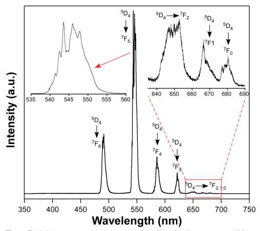
**Figure 7.** 10 K emission spectrum of compound **1** collected under excitation at 325 nm showing the characteristic transitions of the corresponding lanthanide (III) ion.
