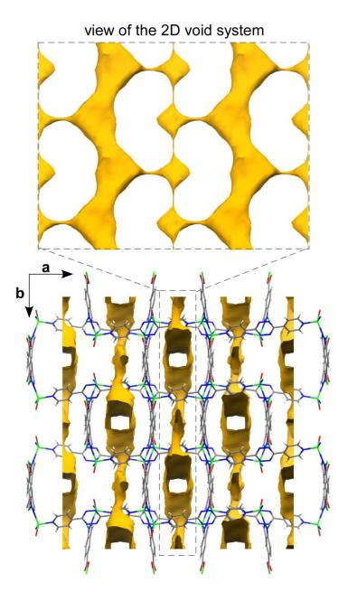
Figure 4. Perspective view of compound 1 showing the solvent-accessible surface.
