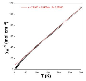
**Figure 11.** *Curie-Weiss fitting (red line) of*  $\chi_M^{-1}$  *vs T (* $^{\circ}$ *) curve.*
