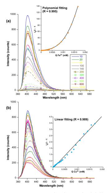
**Figure 11.** Luminescence quenching of  $H_2O@3$  with gradual addition (microliters of metal ion solutions added are shown in the capture with different colours of (a) Fe<sup>3+</sup> and (b) Cu<sup>2+</sup> ions. Stern-Volmer plots showing the best fits are also shown.
