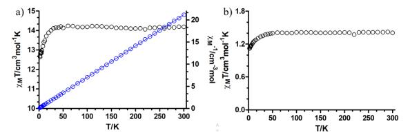
**Figure 4.** a) Temperature dependence of the  $\chi_M T$  product and  $1/\chi$  versus T for 1 in the 2-300 K range. The solid line represents the best fitting with the Curie-Weiss law. b) Temperature dependence of the  $\chi_M T$  product for  $\mathbf{1}_Y$  in the 2-300 K range.
