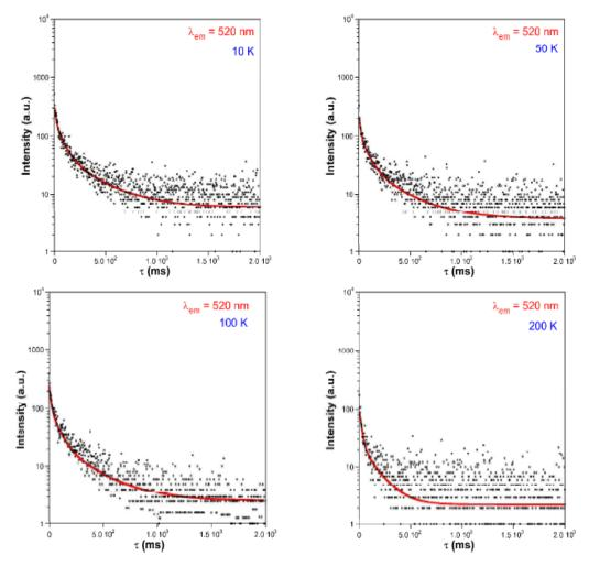
**Figure 19.** Variable-temperature decay curves at  $\lambda_{ex} = 325$  nm and  $\lambda_{em} = 520$  nm showing the best fitting.
