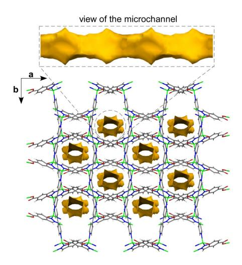
Figure 7. Perspective view of compound 2 showing the solvent-accessible surface. Colour code: zinc, light steel blue; oxygen, red; nitrogen, blue; carbon, grey; chloride, green.
