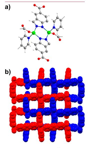
**Figure 1.** Crystal structure of compound 1: (a) fragment containing the SBU and (b) perspective view showing the perpendicular disposition of the pillaring pbptz linkers with regard to the  $Zn/(5-inca)^{2-}$  layers. Color code: zinc, green; oxygen, red; nitrogen, blue; carbon, gray; hydrogen, white.
