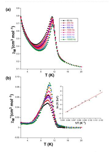
**Figure 5.** Temperature dependence of the (a)  $\chi_M'$  and (b)  $\chi_M''$  signals for compound 1 under an applied field of 1000 Oe. Inset shows the Arrhenius plot with the linear fitting to estimate the thermal barrier for the reversal of the magnetization.
