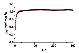
**Fig. 5.** Temperature dependence of the  $\chi_M T$  product for compound 1 in the 2.5–300 K range. The solid line is generated from the best fit to the magnetic parameters.
