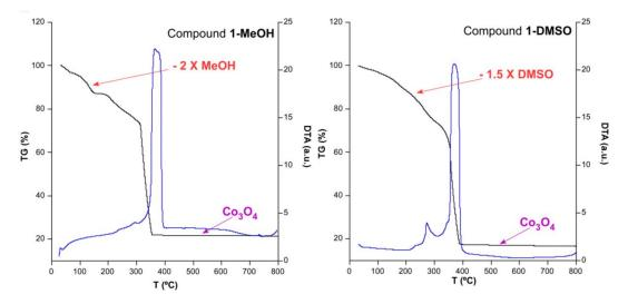
Figure 11. TG/DTA analysis forsolvent exchanged compounds 1-MeOH and 1-DMSO.
