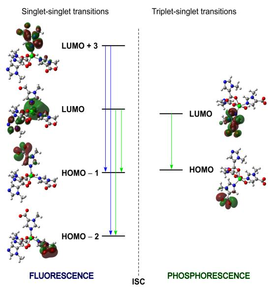
Figure 18. Energy diagram of the orbitals onto model 4 involved in the electronic transitions of 4 resulting in fluorescent and phosphorescent blue and green emissions. ISC: Intersystem crossing.
