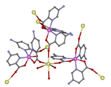
**Figure 3.** Perspective of one chain pertaining to Co-CP in which  $[Co(ampy)_3]^-$  units are connected by  $K^+$  ions. Hydrogen atoms have been omitted for clarity. Colour code: Cobalt, pink; potassium, yellow; oxygen, red; nitrogen, blue; carbon, grey.
