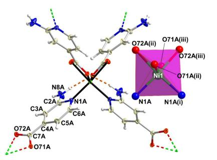
**Figure 1.** Fragment of crystal structure of compound **2** showing labelling mode and the distorted octahedral coordination environment. Connectivity of the structure is inferred by dashed double-colour lines whereas dashed orange lines stand for hydrogen bonds.
