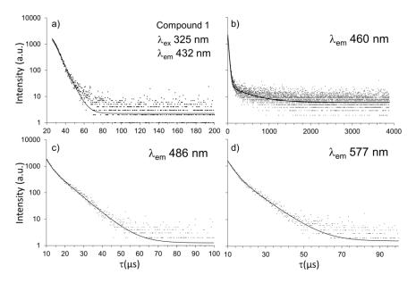
**Figure 11.** Luminescence decay curves for main transitions in 1 (50 K,  $\lambda_{ex}$ =325 nm).
