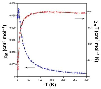
**Figure 12.** *Magnetic susceptibility*  $\chi_M vs T$  ( $\circ$ ) *and*  $\chi_M T vs T$  ( $\Box$ ) *curves of compound* **3** *with best fitting* (-).
