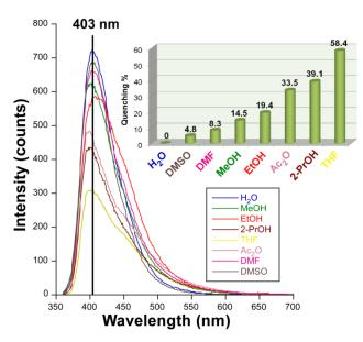
Figure 19. Quenching capacity of solvents based on the emission intensity of 3 under maximum excitation wavelength.
