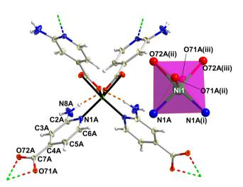
**Figure 1.** Fragment of crystal structure of compound **2** showing labelling mode and the distorted octahedral coordination environment (inset). Connectivity of the structure is inferred by dashed double-colour lines whereas dashed orange lines stand for hydrogen bonds.
