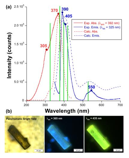
**Figure 7.** (a) Room temperature excitation (red) and emission (blue) spectra of compound **3** showing the most relevant experimental maxima (circles) and calculated (TD-DFT) main vertical excitations (green lines). (b) Micro-PL photographs of a single crystal of **3** illuminated with different lights.
