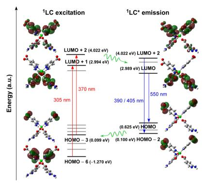
**Figure 8.** Schematic representation of the most intense excitation (red) and emission (blue) lines of compound **3** with their corresponding MOs. Values given between brackets represent the energies.
