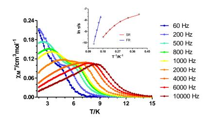
**Figure 9.** Temperature dependence of the molar out-of-phase ac magnetic susceptibility  $(\chi_M")$  for **2** under an applied field of  $H_{dc} = 1000$  Oe at different frequencies. Inset: Arrhenius plot (blue and red lines) for the relaxation times.
