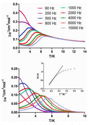
**Fig. 8.** Temperature dependence of in-phase (top) and out-of-phase (bottom) components of the ac susceptibility measured under 1000 Oe applied dc field for **3**. Inset: Arrhenius plots for the relaxation times.
