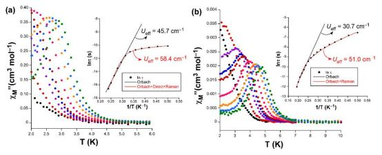
**Figure 12.** Temperature dependence of the  $\chi_M$ " signals and best fitting results for the relaxation times for compounds (a) **1-DMSO** and (b) **1-MeOH**.
