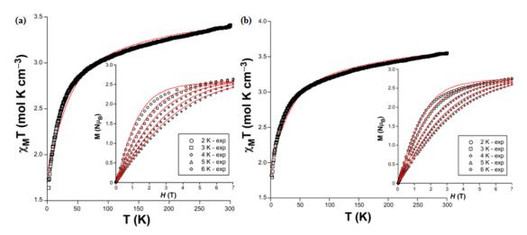
**Figure 14.** Variable temperature  $\chi_M T$  vs Tand M vs H plots with best fitting for (a) **1-DMSO** and (b) **1-MeOH** under an applied field of 1000 Oe.
