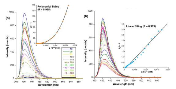
**Figure 24.** Luminescence quenching of  $H_2O@3$  with gradual addition (microliters of metal ion solutions added are shown in the capture with different colors of (a)  $Fe^{3+}$  and (b)  $Cu^{2+}$  ions. Stern-Volmer plots showing the linear fits are also shown.
