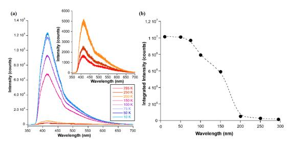
**Figure 18.** (a) Variable temperature emission spectra of **3** under excitation at 305 nm. (b) Evolution of the integrated intensity of the emission according to temperature.
