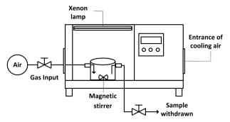
Scheme II. Experimental set-up for photocatalytic experiments.
