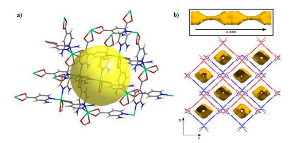
Figure 3. a) Fragment of the structure of compound 2 showing the potential void (sphere of ca. 8 Å diameter) left by the crystallization of one subnet. b) Crystal packing of compound 2 showing the two-fold interpenetrated structure and the microchannels.
