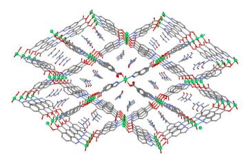
Fig. 3. View of the channels in network compound 1 along a axis showing the crystallization DMF molecules. Hydrogen atoms have been omitted for clarity.
