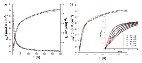
**Figure 7.** (a)  $\chi_M$  and  $\chi_M T$  vs T plots of 1 with best fit according to eq 2. (b) Simultaneous fitting of the  $\chi_M T$  vs T and M vs H plots using eq 3.
