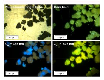
Figure 8. Room temperature micro-PL images for single crystals of compound 2.
