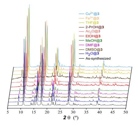
Figure 22. PXRD data of as-synthesized sample and samples collected after suspensions.
