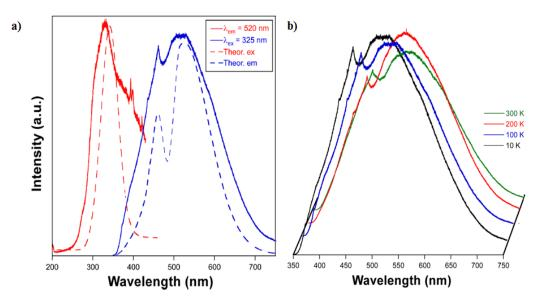
Figure 15. (a) Experimental (solid line) and calculated (dotted line) excitation and emission spectra of compound 4. (b) Variable-temperature emission spectra of compound 4.
