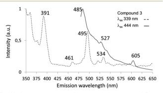
Fig. 11 Room temperature solid state emission spectra of 3 upon sample excitation with a laser,  $\lambda_{ex} = 339$  nm (dashed line) or  $\lambda_{ex} = 444$  nm (solid line).
