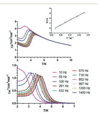
**Fig. 5** Temperature dependence of in-phase (top) and out-of-phase (bottom) components of the ac susceptibility of compound **1** measured under 1000 Oe dc field. Inset: Arrhenius plots for the relaxation times. The black line corresponds to the best fits to the Orbach process.
