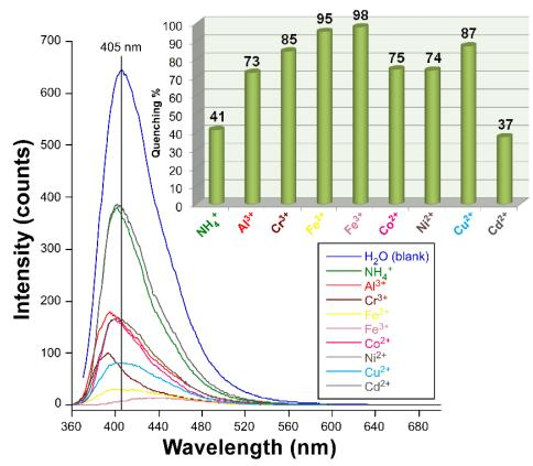
**Figure 23.** *PL response of*  $H_2O@3$  *against common metal ions* ( $\lambda_{ex} = 350$  nm) *together with the quenching percentage estimated from the maximum emission intensity respect to a blank solution.*
