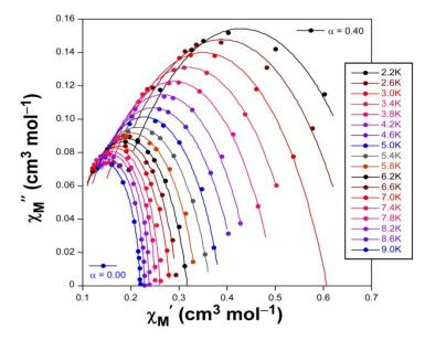
Figure 14. Cole-Cole plot for compound 2 under an applied dc field of 1 KOe.
