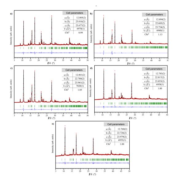
Figure 26. a) Full profile pattern-matching analysis of 1. b) Full profile pattern-matching analysis of 2. c) Full profile pattern-matching analysis of 3. d) Full profile pattern-matching analysis of 1-DMSO. e) Full profile pattern-matching analysis of 1-MeOH.
