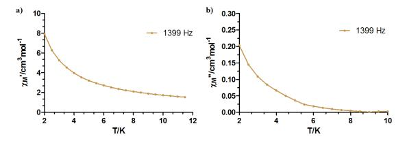
Figure 6. Temperature dependence in-phase (a) and out-of-phase (b) components of the ac susceptibility in a zero applied dc field for 1.
