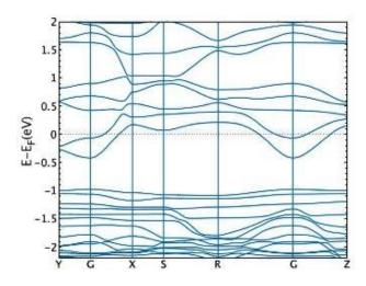
Figure 9. Band structure for 3D material upon replacement of 1:4 oxygend with a hydrogen atom.
