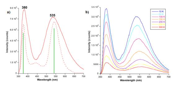
**Figure 13.** *a)* Comparison between room temperature experimental and calculated emission spectra of compound **2**. Black numbers and green lines represent the main experimental emission maxima and calculated vertical main lines, respectively. *b*) Emission spectra of compound **2** monitored under  $\lambda_{ex} = 325$  nm recorded at different temperatures.
