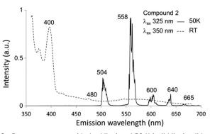
**Fig. 9** Room temperature (dashed line) and 50 K (solid line) solid state emission spectra of **2** upon sample excitation with a laser beam of  $\lambda_{ex}$  = 350 nm and  $\lambda_{ex}$  = 325 nm, respectively.
