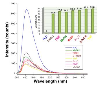
**Figure 9.** PL emission spectra of dispersion of compound **3** in different solvents at their maximum excitation wavelength. Inset shows quenching percentage estimated from the emission intensity relative to  $H_2O@3$  is reflected in the upper bar chart.
