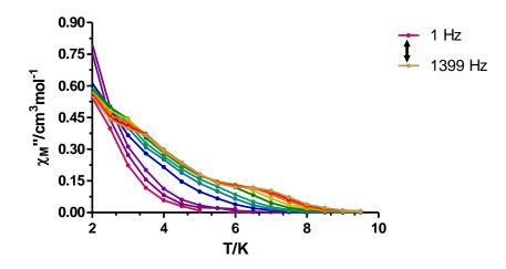
Figure 7. Temperature and frequency dependence of the out-of-phase ac susceptibility of 1 under an external dc field of 1 kOe.
