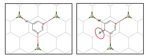
**Scheme I**. Design of 2D-MOF by using 4-hydroxypyrimidine-5-carbonitrile and copper metal ions.
