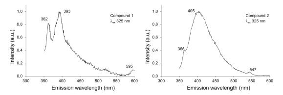
Figure 16. Room temperature emission spectra of water solutions of 1 (left) and 2 (right)  $(\lambda_{ex}=325 \text{ nm})$ . The emission spectra revealed that luminescent processes in 1 or 2, involving the central metal cations, are largely quenched in solution; in this respect, a weak band is observed centered at ca. 595 nm in 1 and ca. 547 nm in 2, which are negligible compared to the ligand derived emission bands observed at shorter wavelengths.
