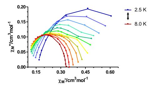
Figure 10. Cole-Cole plots in a dc applied field of 1000 Oe for 1. Solid lines represent the best fitting of the experimental data to the Debye model.
