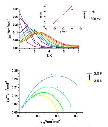
**Fig. 5.** Temperature and frequency dependence of the out-of-phase ac susceptibility of  $\mathbf{1}_{\mathbf{Y}}$  under an external dc field of 1 kOe (top), Arrhenius plot of relaxation time *versus* temperature for  $\mathbf{1}_{\mathbf{Y}}$  (the solid line represents the best fit to the Arrhenius law, top inset) and Cole-Cole plots of  $\mathbf{1}_{\mathbf{Y}}$  under 1 kOe dc field in the temperature range of 2.0–3.5 K (solid lines are the best fit to the generalized Debye mode, bottom).
