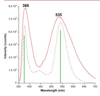
**Figure 7.** Comparison between room temperature experimental and calculated emission spectra of compound **2**. Black numbers and green lines represent the main experimental emission maxima and calculated vertical main lines, respectively.
