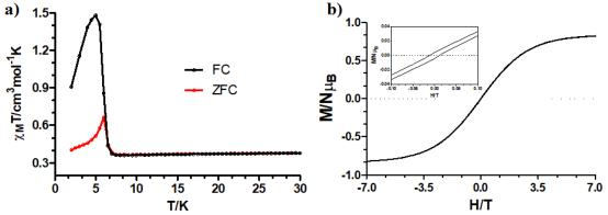
**Figure 8.** *a*)*ZFC and FC curves at* H = 100 *Oe. b*) *Hysteresis loop measured at 2 K in the*  $\pm 7$  *T range.*
