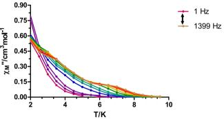
Fig. 4. Temperature and frequency dependence of the out-of-phase ac susceptibility of 1 under an external dc field of 1 kOe.
