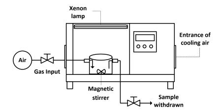
Scheme I. Experimental set-up for photocatalytic experiments.
