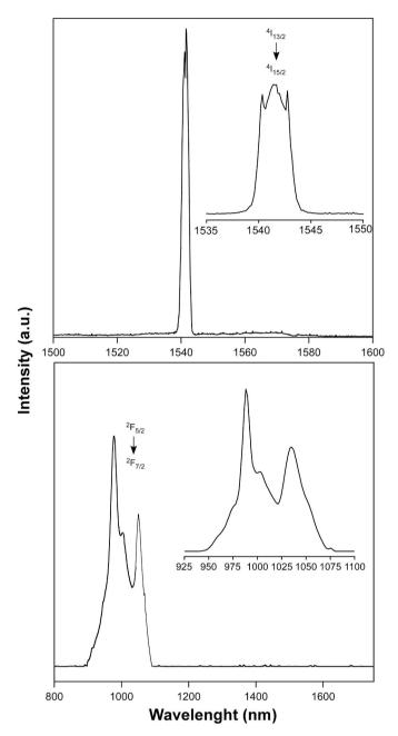
Fig. 7. 10 K emission spectra of compounds 2 and 3 collected under excitation at 325 nm showing the characteristic transitions of the corresponding lanthanide(III) ion.
