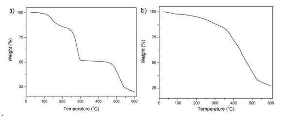
**Figure 2.** (a) Thermogravimetric analysis (TGA) profile of **1** at a heating rate of 5 °C/min under a constant stream of N<sub>2</sub>. (b) Thermogravimetric analysis (TGA) profile of **2** at a heating rate of 5 °C/min under a constant stream of N<sub>2</sub>
