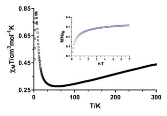
**Fig. 6.** Temperature dependence of the  $\chi_M T$  product for compound **2** in the 2–300 K range. Inset: field dependence of the magnetization for **2**.
