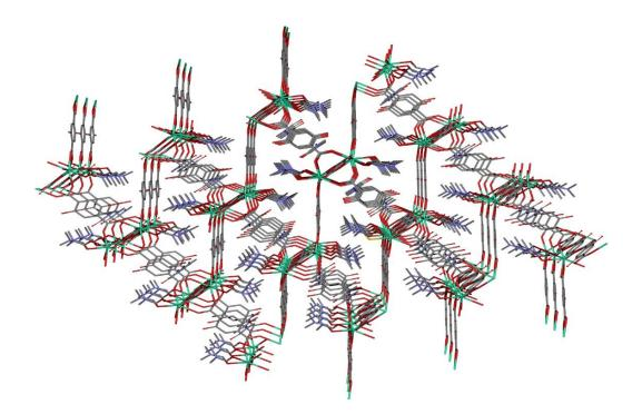
Figure 3. Perspective of Metal-Organic Framework along a axis.Colour code: dysprosium, oxygen, nitrogen and carbon are in light green, red, blue and grey, respectively. Hydrogen atoms have been removed for the sake of clarity.
