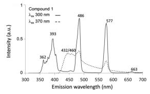
Fig. 7 Room temperature solid state emission spectra of 1 upon sample excitation at  $\lambda_{ex}$  = 300 nm (solid line) and  $\lambda_{ex}$  = 370 nm (dashed line).
