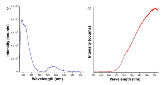
**Figure 16**. (a) Emission spectrum of compound **3** under excitation at 370 nm. (b) Excitation spectrum of compound **3** monitored under  $\lambda_{em} = 550$  nm.
