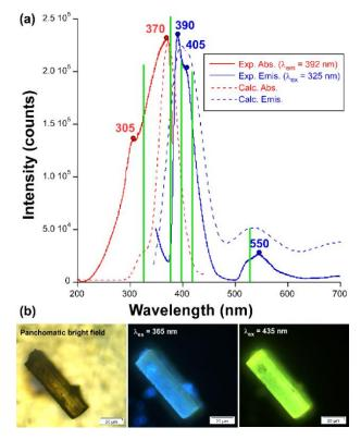
Figure 15. (a) Room temperature excitation (red) and emission (blue) spectra of compound 3 showing the most relevant experimental maxima (circles) and calculated (TD-DFT) main vertical excitations (green lines). (b) Micro-PL photographs of a single crystal of 3 illuminated with different lights.
