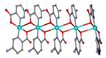
**Fig. 5.** Perspective of one chain pertaining to Cu-CP parallel to *a* axis. Hydrogen atoms have been omitted for clarity. Colour code: Copper, cyan; oxygen, red; nitrogen, blue; carbon, grey. (For interpretation of the references to colour in this figure, the reader is referred to the web version of this article.)
