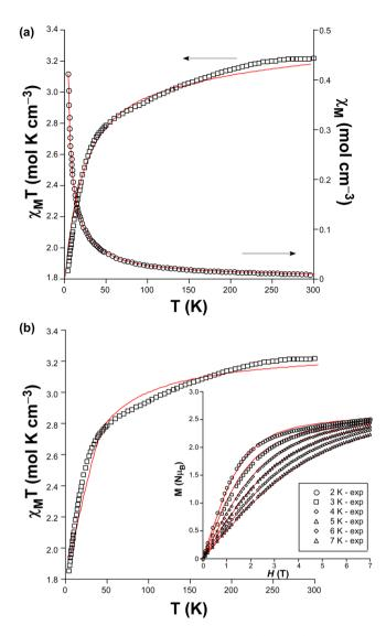
**Figure 3.** (a)  $\chi_M$  (o) and  $\chi_M T$  ( $\Box$ ) vs *T* plots of 1 with best fit according to Eq. 2. (b) Simultaneous fitting of the  $\chi_M T$  vs *T* and *M* vs *H* (inset) plots using Eq. 3.
