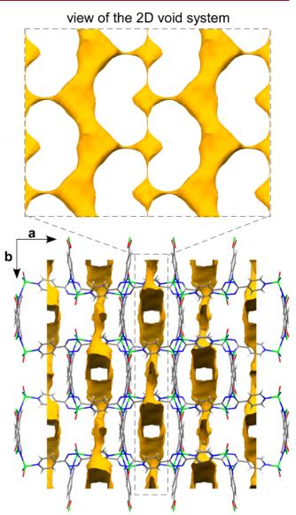
Figure 2. Perspective view of compound 1 showing the solvent-accessible surface.
