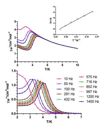
Figure 7. Temperature dependence of in-phase (top) and out-of-phase (bottom) components of the ac susceptibility of compound 1 measured under 1000 Oe dc field. Inset: Arrhenius plots for the relaxation times. The black line corresponds to the best fits to the Orbach process.
