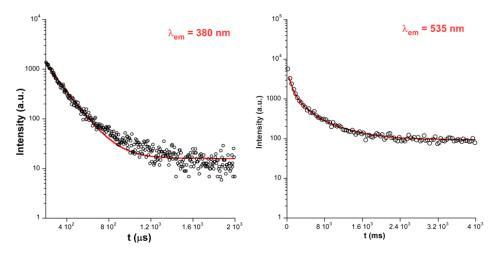
**Figure 15.** Decay curves with best fitting at room temperature for compound 2 ( $\lambda_{ex} = 325$ ).
