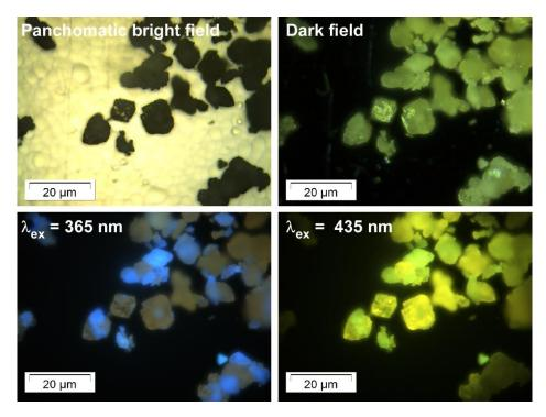
Figure 17. Room temperature micro-PL images for single-crystals of compound 2.
