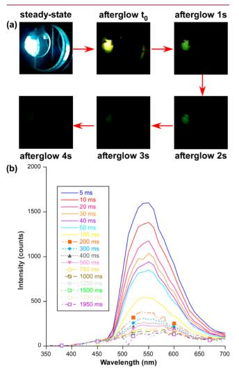
**Figure 9.** (a) Photographs of the steady-state and afterglow emissions of compound 2. (b) TRES of compound 2 at 10 K at selected delays ( $\lambda_{ex}$  = 325 nm).
