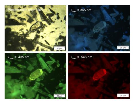
Figure 18. Micro-PL images taken on single crystals of 2.
