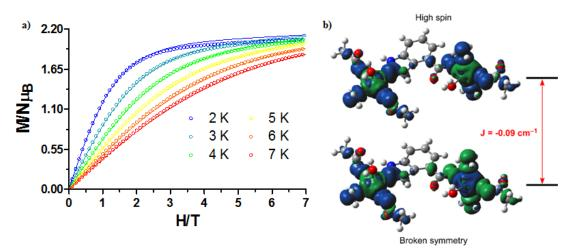
Figure 5. a) Field dependence of the magnetization for 1. The solid lines are generated from the best fit to the magnetic Parameters. b) Broken-symmetry DFT based calculation on 1 (top) and 3 (down) to account for the value of the exchange parameter. Spin densities are shown for ground and excited states involving the superexchange pathway.
