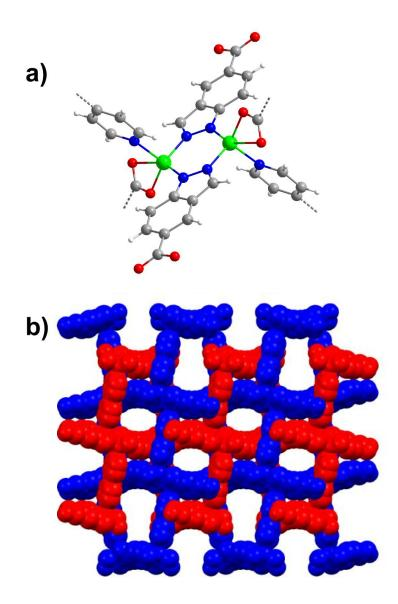
**Figure 6.** *a)* SBU of the structure of compound 2 and b) crystal packing of the compound showing the two-fold interpenetration.
