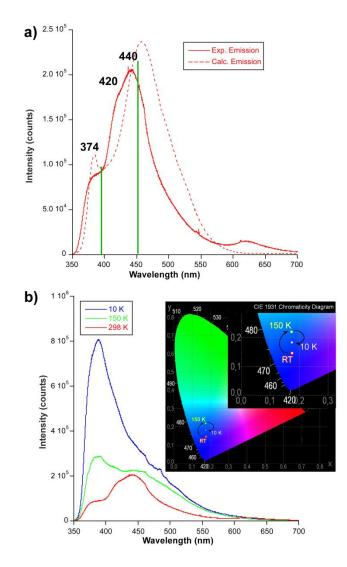
Figure 8. a) Room temperature experimental (solid red line) and TD-DFT calculated (dotted red line) steady-state emission spectra of compound 1. Black numbers account for experimental emission maxima whereas main calculated main lines are represented as vertical green lines. b) Experimental emission spectra of 1 at variable temperature together with the thermochromic emission. Inset shows luminescent thermochromism represented in the CIE1931 chromaticity color coordinates.
