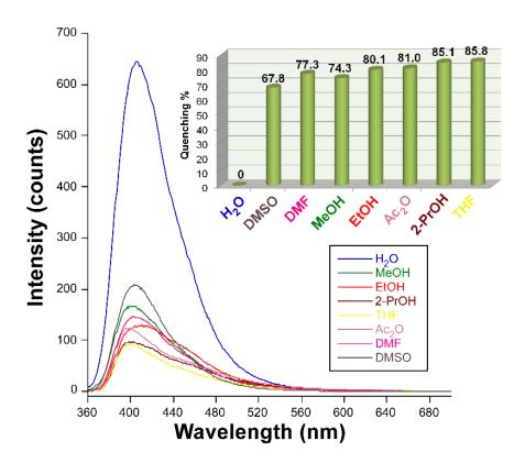
Figure 21. PL emission spectra of dispersion of compound 3 in different solvents at their maximum excitation wavelength. Quenching percentage estimated from the emission intensity relative to  $H_2O@3$  is reflected in the upper bar chart.
