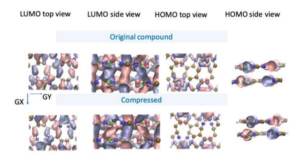
. Figure 7. Wavefunction spatial distribution in the G point for the lowest unoccupied and highest occupied states. Copper, carbon, oxygen, nitrogen and hydrogen atoms are displayed in green, brown, red, blue and white, respectively. The arrows indicate the direction of the GX and GY paths in the reciprocal space.
