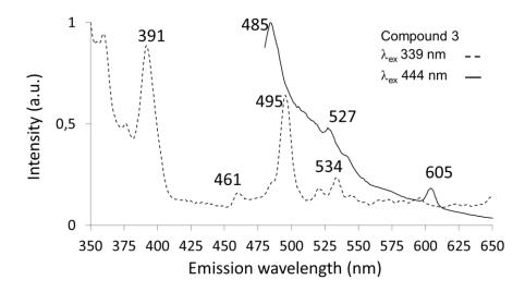
**Figure 14.** Room temperature solid state emission spectra of **3** upon sample excitation with a laser of  $\lambda_{ex}$ = 339 nm (dashed line) or of  $\lambda_{ex}$ = 444 nm (solid line).
