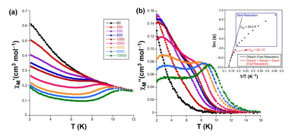
**Figure 13.** Temperature dependence of (a) in-phase and (b) out-of-phase ac magnetic susceptibilities under an applied field of 1000 Oe for compound **2**. Inset: Arrhenius plot of relaxation times with best fittings
