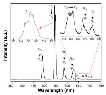
Fig. 6. 10 K emission spectrum of compound 1 collected under excitation at 325 nm showing the characteristic transitions of the corresponding lanthanide (III) ion.
