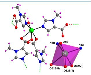
**Figure 6.** Relative disposition of square rings within the layer, hydrogen-bonding interactions between layers, and their mutual packing in compound **4**.
