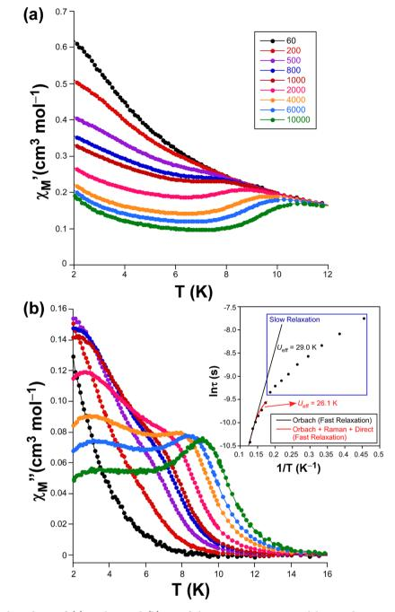
Figure 9. Temperature dependence of (a) in-phase and (b) out-of-phase ac magnetic susceptibilities under an applied field of 1000 Oe for compound 2. Inset: Arrhenius plot of relaxation times with best fittings.
