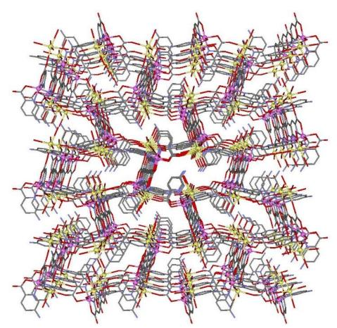
Figure 4. Perspective of the three-dimensional structure in Co-CP. Hydrogen atoms have been omitted for clarity. Colour code: Cobalt, pink; potassium, yellow; oxygen, red; nitrogen, blue; carbon, grey.
