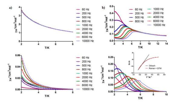
Figure 9. a) Temperature dependence of in-phase (top) and out-of-phase (bottom) components of the ac susceptibility measured under 1000 Oe applied dc field for 2. b) Temperature dependence of in-phase (top) and out-of-phase (bottom) components of the ac susceptibility measured under 1000 Oe applied dc field for 3. Inset: Arrhenius plots for the relaxation times. The black and red lines correspond to the best fits to Orbach and Raman + QTM processes, respectively.
