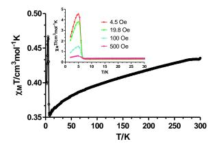
**Figure 7.** Temperature dependence of the  $\chi_M T$  product for **3** in the 2-300 K range. Inset: temperature dependence of the  $\chi_M T$  product at the indicated fields in the 2-30 K range.
