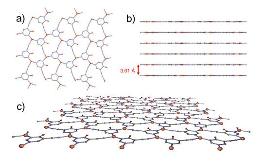
**Figure 2.** *a)* Perspective of 2D plane in MOF. b) Separation among sheets in MOF. c) Projection in perspective of MOF.
