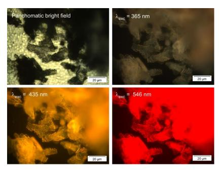
Figure 17. Micro-PL images taken on single crystals of 1.
