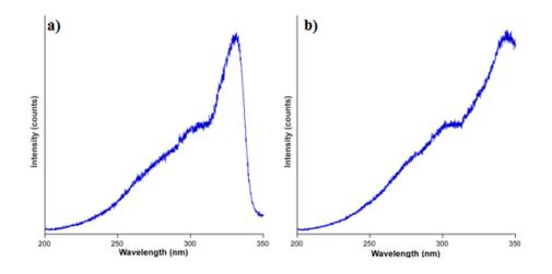
**Figure 10.** *Excitation spectra of compound* **2** *monitored under* (*a*)  $\lambda_{em} = 380$  nm and (*b*)  $\lambda_{em} = 535$  nm.
