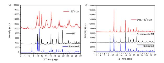
**Figure 1.** (a) Powder X-ray diffraction patterns of simulated, experimental and desolvated sample (2h at 150 °C) of **1**. (b) Powder X-ray diffraction patterns of simulated, experimental and desolvated sample (2h at 150 °C) of **2**.
