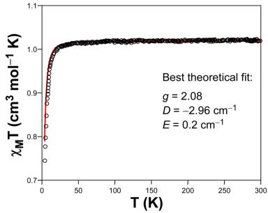
**Figure 9.** *Fitting (red line) of*  $\chi_M Tvs T$  ( $\circ$ ) *curve of compound 1.*
