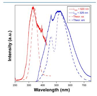
Figure 10. Experimental (solid line) and calculated (dotted line) excitation and emission spectra of compound 4.
