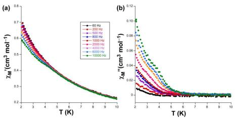
**Figure 9.** Temperature dependence of the (a)  $\chi_M$ ' and (b)  $\chi_M$ '' signals for compound **1** with no applied dc field.
