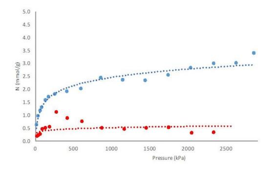
Figure 5. Carbon dioxide adsorption at 273 K on Compound 2 (blue) and 1 (red). Trend lines are just guides for eyes.
