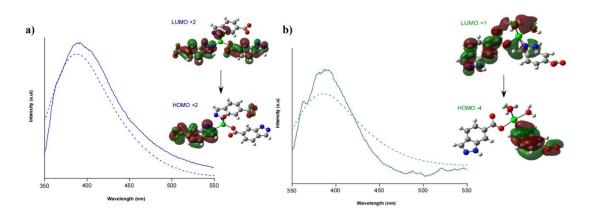
**Figure 8.** Room temperature TD-DFT computed (dashed lines) and experimental (solid line) photoluminescence emission under  $\lambda_{ex} = 325$  nm of CPs. Blue and green lines correspond to compound 1 and 2, respectively. The insets show the most representative molecular orbitals involved in the electronic transitions.
