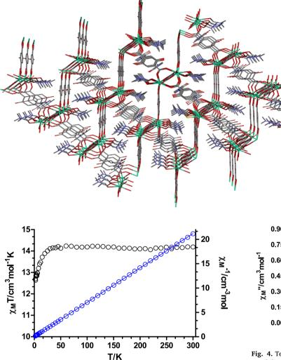
**Fig. 3.** Temperature dependence of the  $\chi_M T$  product and  $1/\chi$  versus *T* for **1** in the 2–300 K range. The solid line represents the best fitting with the Curie-Weiss law.
