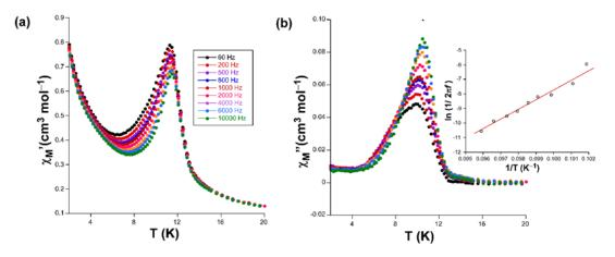
**Figure 10.** Temperature dependence of the (a)  $\chi_M$ ' and (b)  $\chi_M$ '' signals for compound 1 under an applied field of 1000 Oe. Inset shows the Arrenhius plot with linear fitting to estimate the thermal barrier for the reversal of the magnetization.
