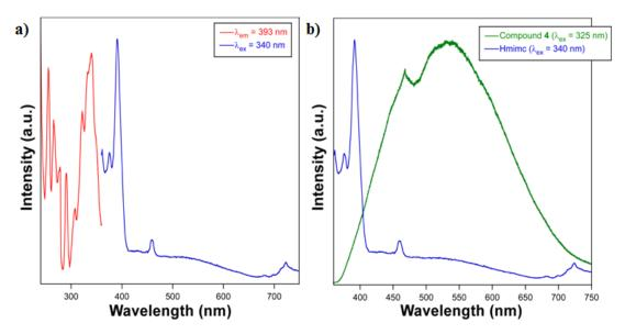
Figure 17. (a) Excitation and emission spectra of Hmimc ligand. (b) Comparison of emission profiles between Hmimc and compound 4.
