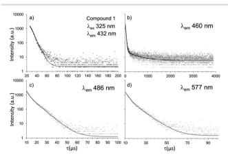
**Fig. 8** Luminescence decay curves for the main transitions in 1 (50 K,  $\lambda_{ex} = 325$  nm). a)  $\lambda_{em} = 432$  nm; b)  $\lambda_{em} = 460$  nm; c)  $\lambda_{em} = 486$  nm; d)  $\lambda_{em} = 577$  nm.
