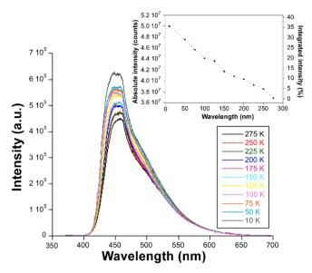
Fig. 9. Variable temperature emission spectra. Inset: evolution of the integrated emission intensity.
