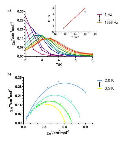
**Figure 8.** Temperature and frequency dependence of the out-of-phase ac susceptibility of  $\mathbf{1}_Y$  under an external dc field of 1 kOe. (a) Arrhenius plot of relaxation time versus temperature for  $\mathbf{1}_Y$  (the solid line represents the best fit to the Arrhenius law, (a) inset). (b) Cole-Cole plots of  $\mathbf{1}_Y$  under 1 kOe dc field in the temperature range of 2.0 - 3.5 K.
