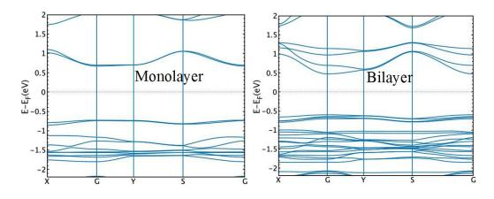
Figure 8. Band structure for an isolated single layer and for two consecutive layers.
