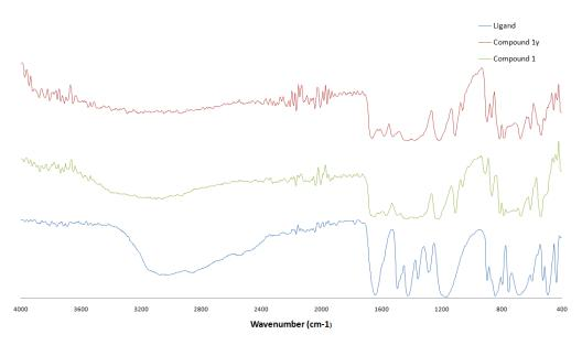
**Figure 1.** The FT-IR spectra of ligand and complexes 1 and  $1_Y$ .
