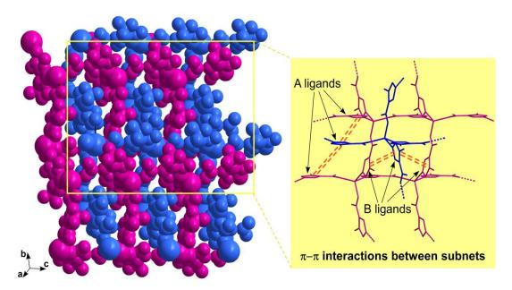
**Figure 4.** View of the 2-fold interpenetrated building of compound 2 (red and blue layers represent independent subnets) showing  $\pi - \pi$  interactions among mimc ligands.
