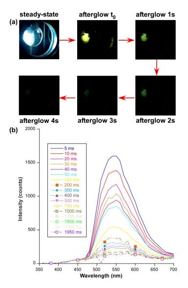
**Figure 19.** (a) Photographs of the steady-state and afterglow emissions of compound 2. (b) TRES of compound 2 at 10 K at selected delays ( $\lambda_{ex} = 325$  nm).
