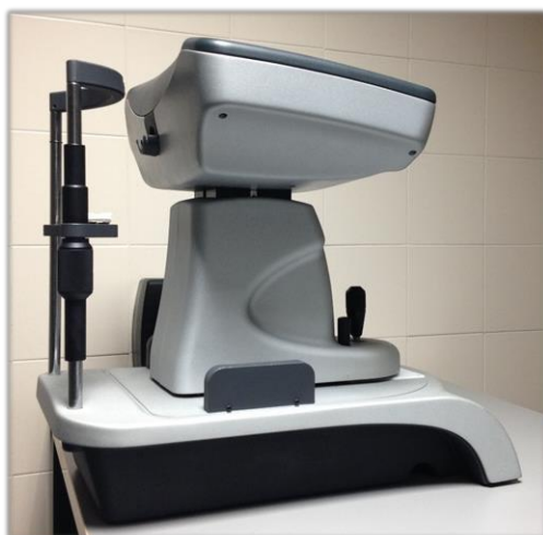
Figura 4.1. OQAS II (Optical Quality Analysis System II, Visiometrics SL).
