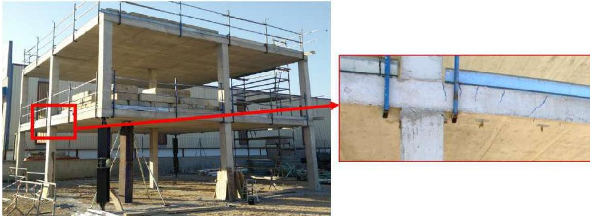
**Figure 10.** Cracks on the slabs near the joint column-slab attached to the failed column after the accidental event in the experimental test.
