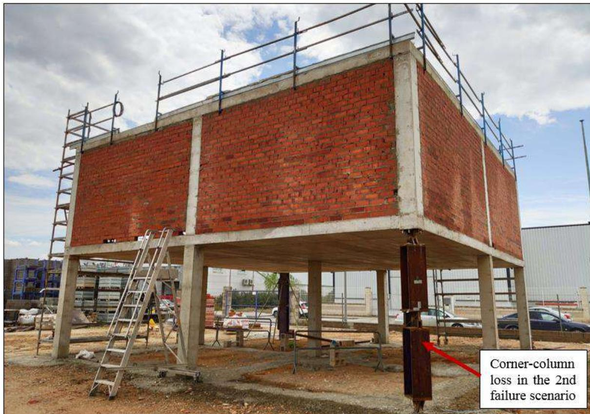
**Figure 4.** Building and definition of the second failure scenario.
