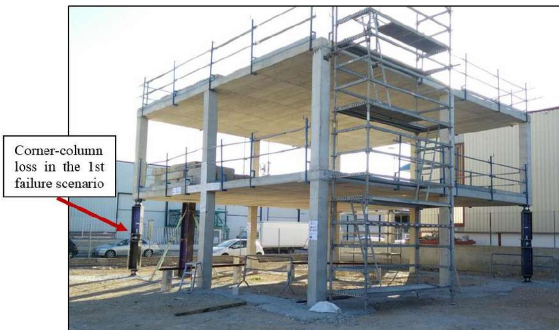
**Figure 3.** Building and definition of the first failure scenario.
