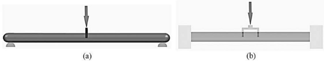
**Figure 3.** Models of pipeline segment with idealized loading conditions: a) simple ends with center-point loading, b) fixed ends with two-point loading
