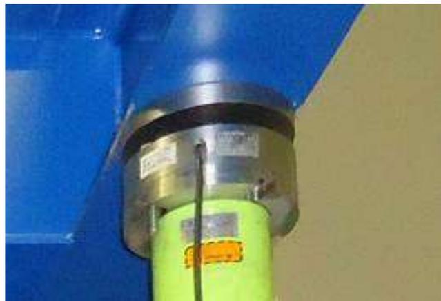
**Figure 4.** *Detail of the load cells.*
