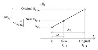
Fig. 7. Correspondence between time intervals and ground acceleration increments to be employed in LAM and computation of new value of  $\ddot{u}_g$  to be introduced in  $\ddot{u}_g$ .
