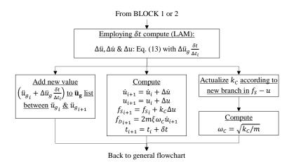
Fig. 10. Block 3 used to recompute the valid values of next iteration variables with the modified time interval  $\delta t$  computed in block 1 or 2.
