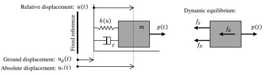
Fig. 1. SDOF system usually employed in earthquake engineering.
