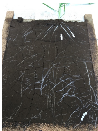
Figure 1. Rhizoboxes used in this study and the average location of the extraction disks during exudate collection.
