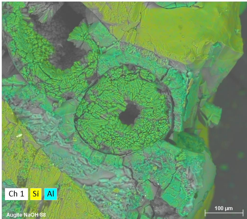
Figure V.3. SEM-EDS compositional map of Figure 2d showing Si (yellow) and Al (Blue). It can be observed that the augite (aug) crystal is fractured after 28 days of reaction and inside the fractures, phillipsite (phi) was precipitated
