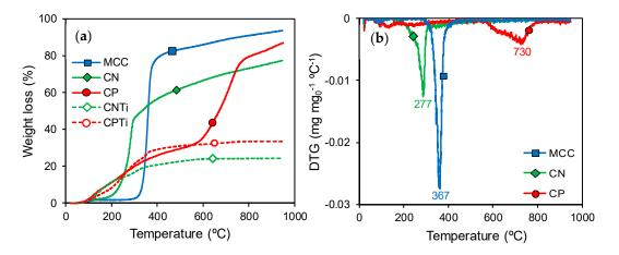
**Figure 1.** (a) Thermogravimetric (TG) profiles under  $N_2$  flow for microcrystalline cellulose (MCC) and acid-treated cellulose samples before (solid lines) and after Ti impregnation (dash lines); (b) Differential thermogravimetric (DTG) profiles under  $N_2$  flow for MCC, CN and CP.
