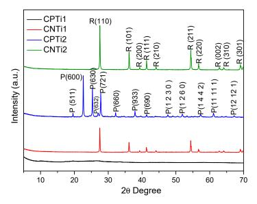
Figure 3. X-ray diffraction (XRD) patterns of the carbon–Ti composites (R = rutile,  $P = TiP_2O_7$ ).
