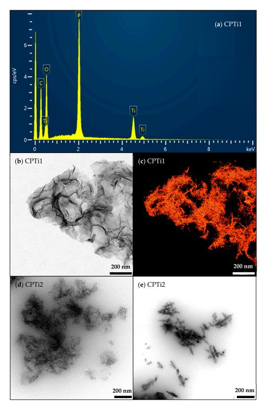
**Figure 5.** High resolution transmission electron microscopy (HRTEM) characterization of CPTi composites: (**a**) energy dispersive X-ray (EDX) analysis, (**b**,**d**,**e**) micrographs and (**c**) Ti-mapping.
