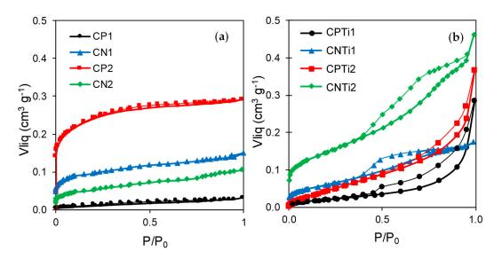
Figure 6.  $N_2$  adsorption-desorption isotherms of (a) the pure carbon materials and (b) the carbon-Ti composites.
