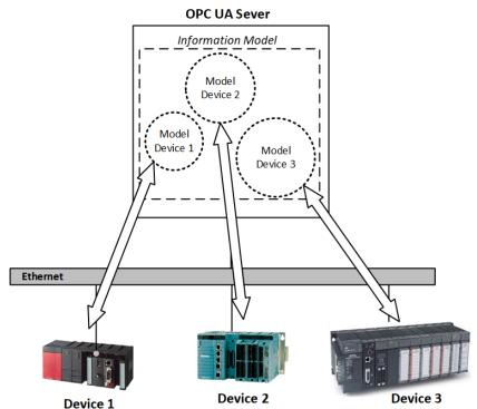
Figure 1. An OPC UA server can manage the information models for each industrial device.
