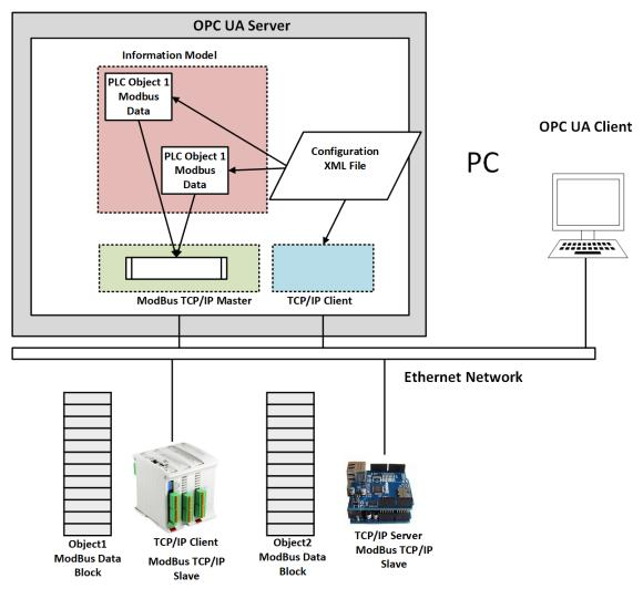
**Figure 5.** Architecture of the system prepared for the case study that includes the OPC UA server, the OPC UA client, the M-DUINO PLC and the Arduino ONE.
