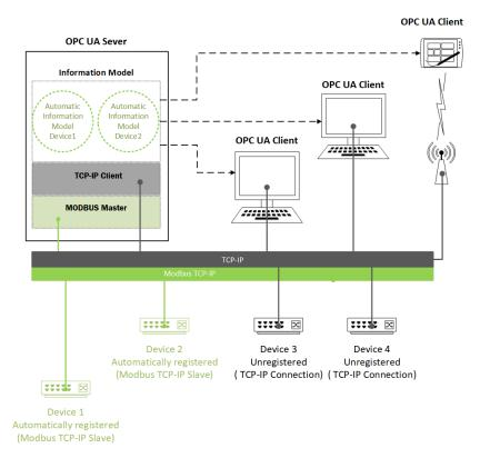
Figure 2. Architecture of the industrial system for the auto-configuration of OPC UA.
