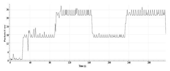
**Figure 10.** The graph includes the network traffic generated between two devices (M-DUINO and Arduino ONE) and the OPC UA server.
