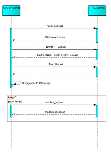
**Figure 3.** Message exchange between the OPC UA server and an industrial device during the auto-configuration of OPC UA server in TCP/IP mode and the subsequent periodic requests/responses in Modbus mode.
