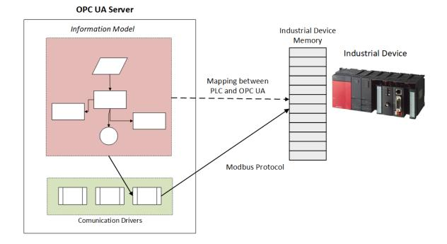
**Figure 4.** Schematic of the information exchange between the PLC device and OPC UA server once the auto-configuration of OPC UA is finished.
