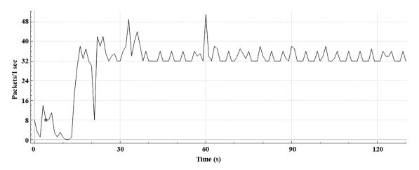
**Figure 11.** The graph includes the network traffic generated between two devices (M-DUINO and Arduino ONE) and the OPC UA sever connected at the same time.
