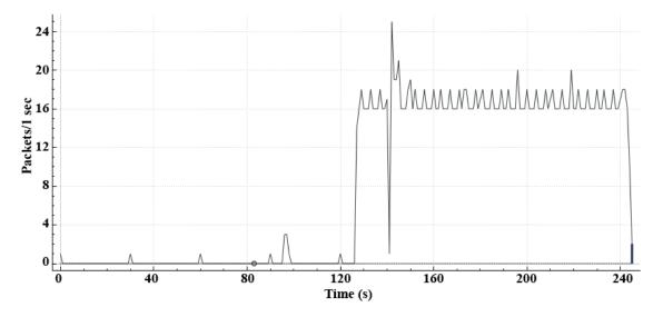
**Figure 9.** The graph includes the network traffic generated between the M-DUINO and the OPC UA server.
