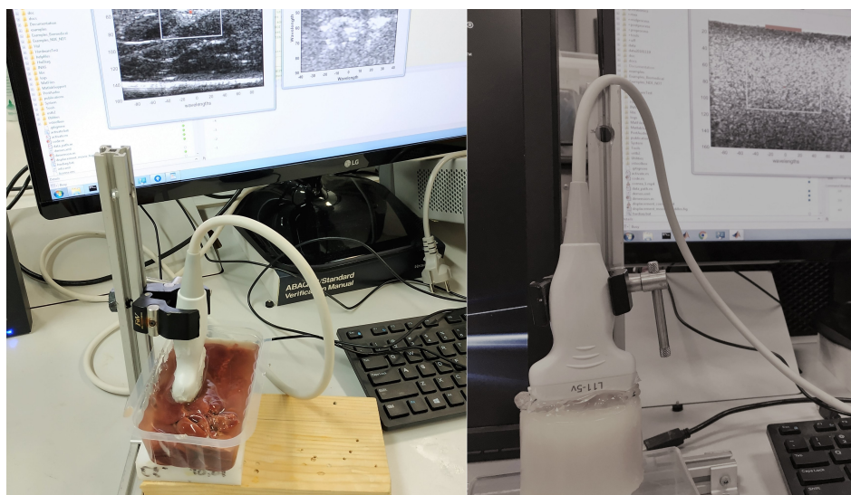
Figure 5. Set-up for measurements using SWEI. The picture was taken during the measurements at the Ultrasonics Lab at the University of Granada. In the left image, the ex vivo liver sample is measured while one of the hydrogel phantoms is shown in the right image.
