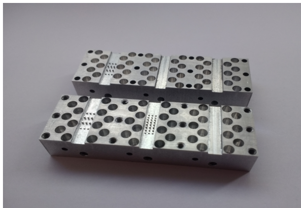
FIGURE 10. CNC milling manufactured prototype.
