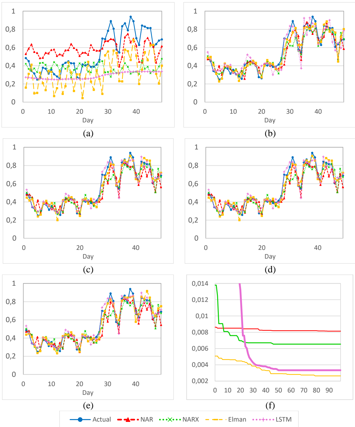
Fig. 11. Example of the optimization process in 100 generations; the model forecasting for the 50-day period in the first generation (a); optimization achieved in Generation 25 (b), in Generation 50 (c), in Generation 75 (d) and the final generation (e); and the mean square error achieved during the process (f) in each generation
