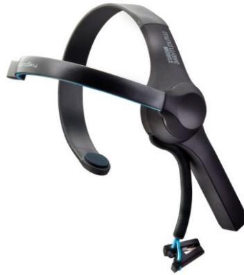
Figure 3.1: NeuroSky MindWave Mobile headset. This device consists of a single dry electrode (12 mm x 16 mm) placed on Fp1, according to the international 10-20 system [88], which inputs data to a TGAM1 (ThinkGear ASIC Module) integrated circuit able to record data at 512 Hz. These two elements are mounted on a light headset (90 g). The device uses a monopolar montage with one active site, and employs a pea-sized ( \sim 0.8 mm diameter) electrode clipped to the left earlobe as reference. Image retrieved from [87].
