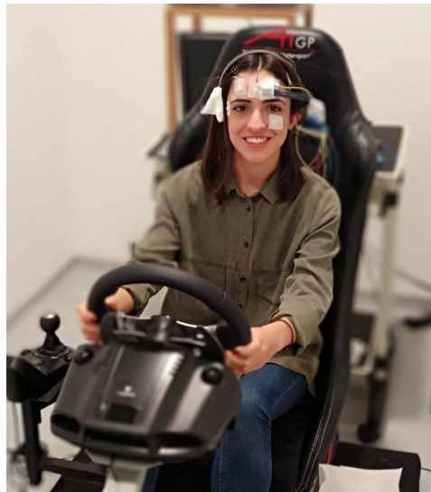
Figure 3.2: Participant wearing simultaneously SOMNOWatch+EEG-6 and NeuroSky MindWave Mobile headset seated in an driving simulator ready to perform the experiment.
