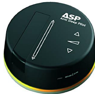
Figure 2.8: Anti Sleep Pilot. The system is placed on the dashboard of the vehicle and from time to time it emits an alarm and counts the time it takes for the operator to press the button. Image retrieved from [86].
