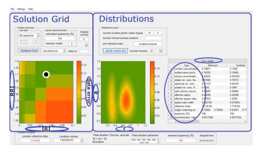
Figure V–2: Screen shot of the SphInX-Main panel, indicating the two main parts: solution grid with the scrutinized *CRI* values and some plot setting options (left), and shape-size distributions and their corresponding particle properties, retrieved in sequence for all selected (s,d) values (right). Adapted from Samaras (2017).
