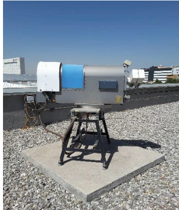
Figure 3.5. Microwave Radiometer (RPG-HATPRO G2, Radiometer physics GmbH) operating at the IISTA-CEAMA station in Granada (Spain).
