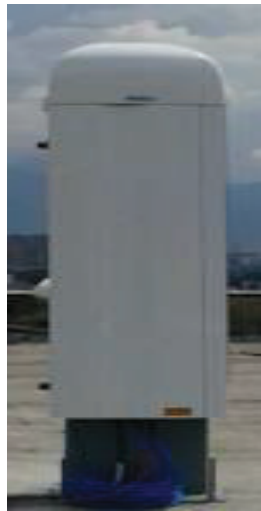
Figure 3.11. Vaisala CL 51 ceilometer located at the roof top of the SIATA-tower..
