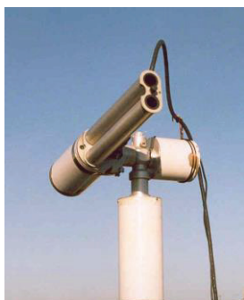
Figure 3.6. Sun/sky photometer (Cimel Electronique) CE-318-4 operating at the IISTA-CEAMA station in Granada (Spain).
