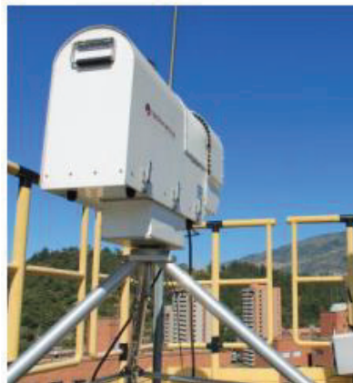
Figure 3.12. Microwave radiometer MP-3000 A located at the SIATA-tower station in Medellín (Colombia).
