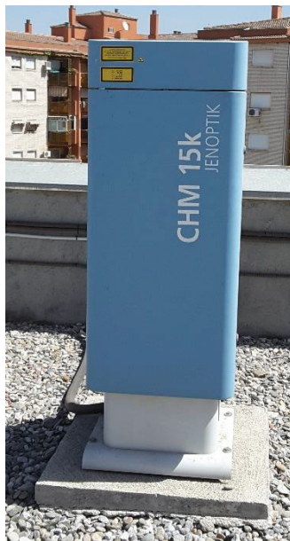
Figure 3 3. Ceilometer CHM15k Jenoptik operating at IISTA-CEAMA station in Granada (Spain).
