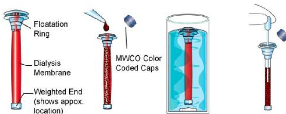
Fig. 1. Float-A-Lyzer dialysis device.
