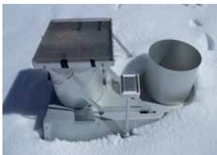
Passive particle collector for wet deposition (left) and dry (right) partially buried in the snow. Multiparametric station of Veleta, Sierra Nevada
