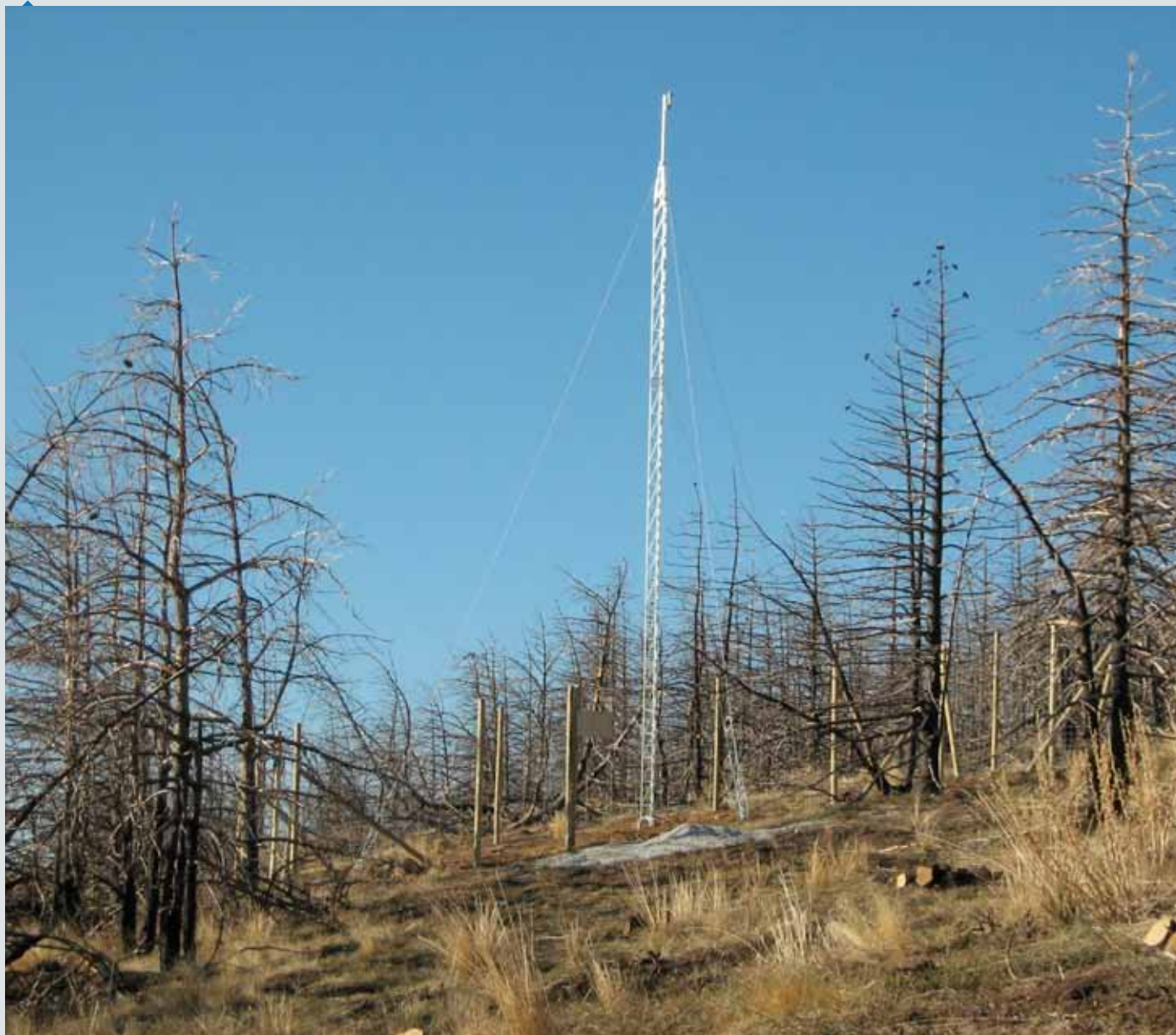
Installation of a monitoring station for carbon fluxes in the areas affected by the fire of Lanjarón.
