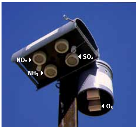
View, from below, of the support for passive dosimeters. A casing holds the collectors of nitrogen dioxide ( \text{NO}_2 ), ammonia ( \text{NH}_3 ), and sulphur dioxide ( \text{SO}_2 ), and the other casing collects ozone ( \text{O}_3 ).
