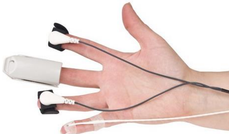
Figure 6. Position of the electrodes to record skin conductance.
