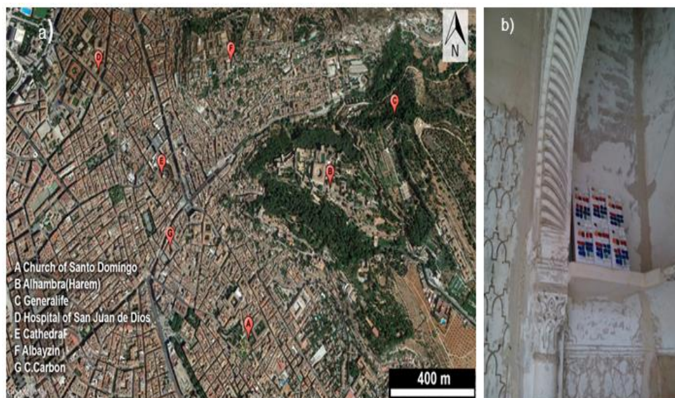
Figure 1. (a) Aerial view of the city of Granada (South Spain) showing the location of the paint dosimeters at (semi)open monuments; (b) set of paint dosimeters placed in the Harem of the Alhambra monument.
