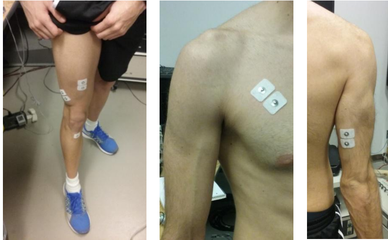
Figure 4.3. Pairs of self-adhesive electrodes (Norotrode 20 TM . Myotronics Inc. Kent, USA) placed according to Kasman (2002) 23 , in Rectus Femoris, Vastus Lateralis, Pectoralis Major, and Triceps Brachii.
