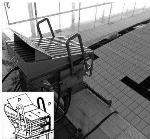
Figure 7.1. Instrumented swimming starting block, replicating OMEGA OSB 12, with its five independent extensometric triaxial force plates (P).
